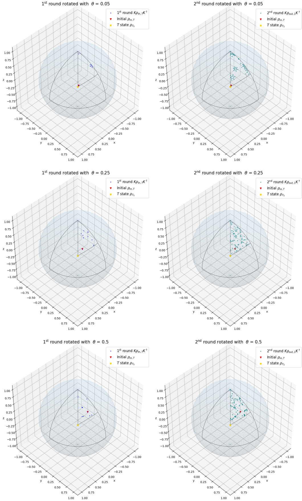
Figure B.4: All the unique states that can be obtained for up to two rounds of optimization and three different initial angles that y rotates the input T states have been plotted on Bloch spheres. Each column is a different round of optimization and each row corresponds to a different rotation angle. The states have been shifted to the same hexant as previous examples.
