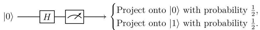
Figure 2.3: An extension of the circuit in Figure 2.2 where the measurement of the output state also is included.
