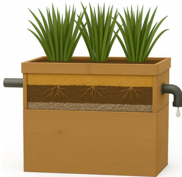
Figure 5.12: Design of the elevated plant filtration bed. The cross section shows the layers of gravel, soil and sand that greywater passes through, as well as the plant roots that treats the water through microbial degradation and plant uptake. The design is based on Collivignarelli et al. (2020).
