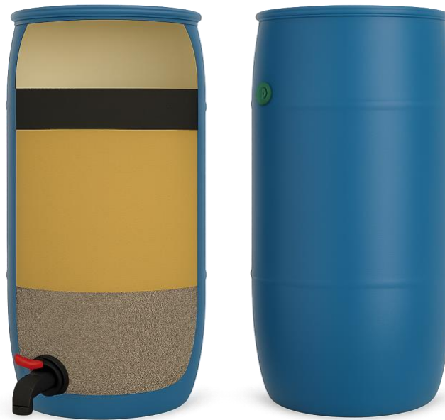
Figure 5.11: Illustration of the greywater treatment barrel. The cross-section shows the gravel, sand, and activated charcoal layers. The design is based on Shaikh & Ahammed (2022) and Huhn et al. (2015).
