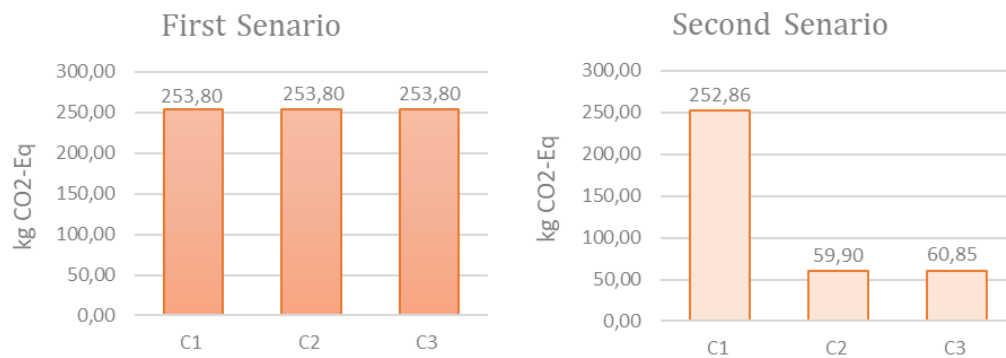
Figure 4.10 Alu+ Polystyrene noise barrier global warming potential (CO 2 kg eq.) in three life cycles (with or without recycling)
