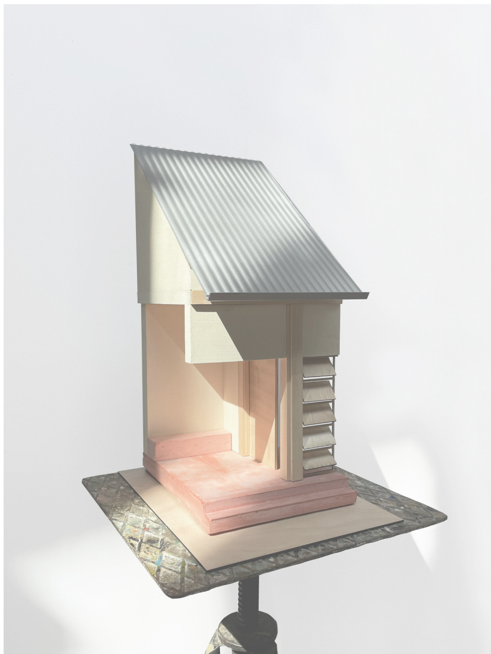
Detail model 1:20 Showing sliding doors in between two-parted pillars
