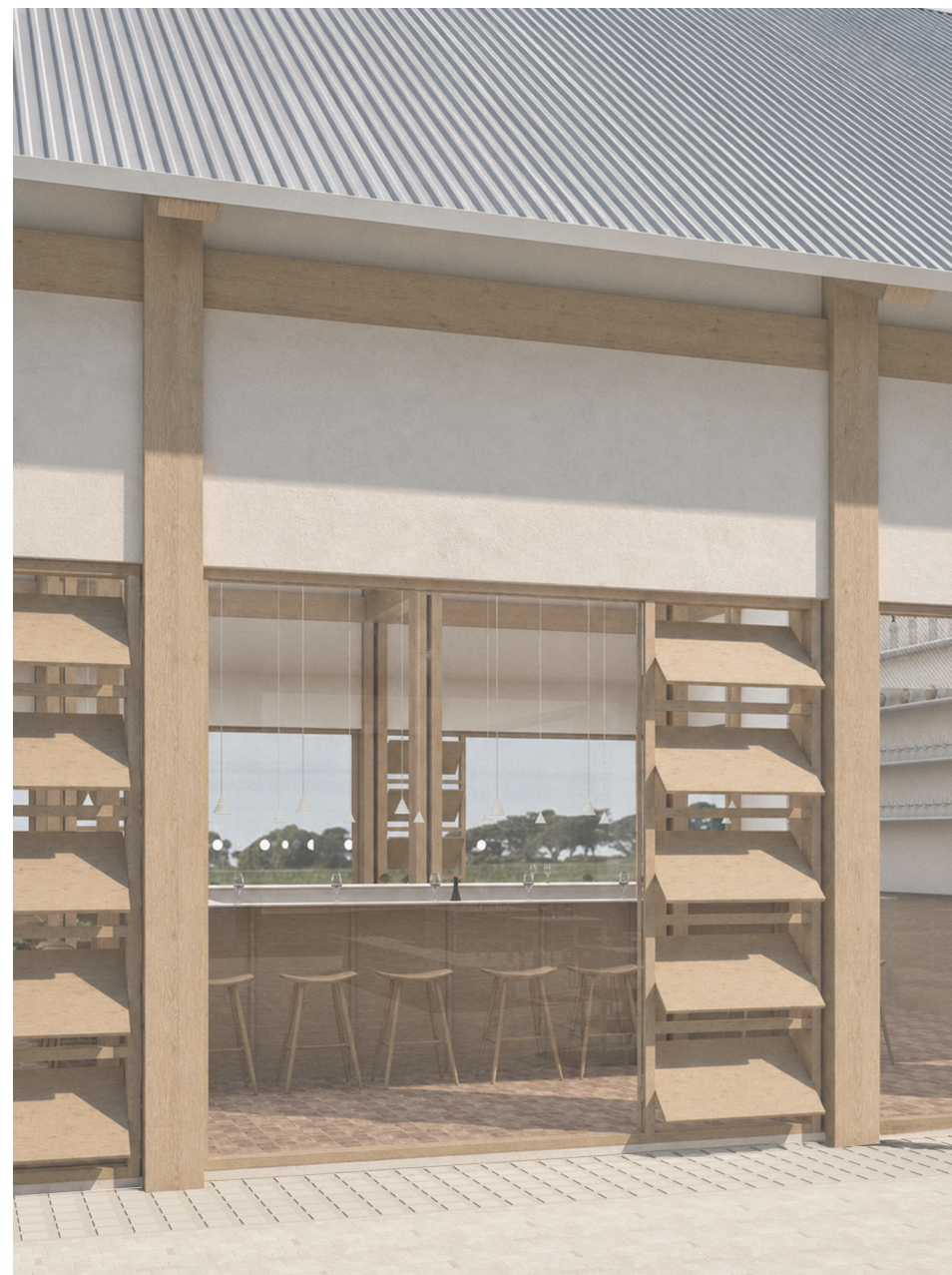
Windows with adjustable wooden slabs for ventilation.
