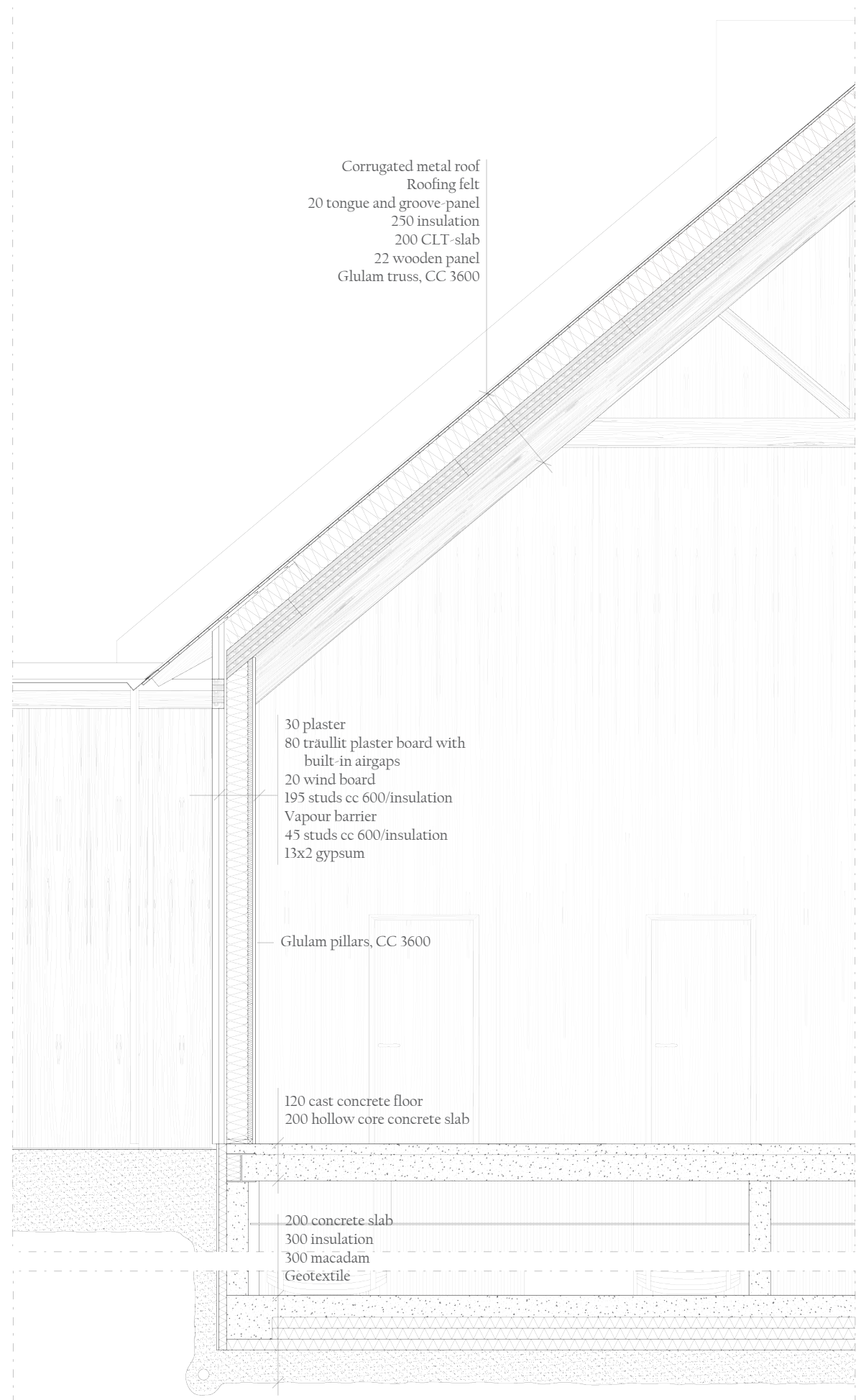
Detail section, production building 1:50 (A4)
