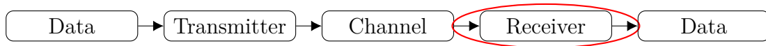
Figure 3.1: Block scheme of Shannon's general communication system. The Receiver block is circled because that is where this thesis aims to make an improvement. Adapted from [14].
