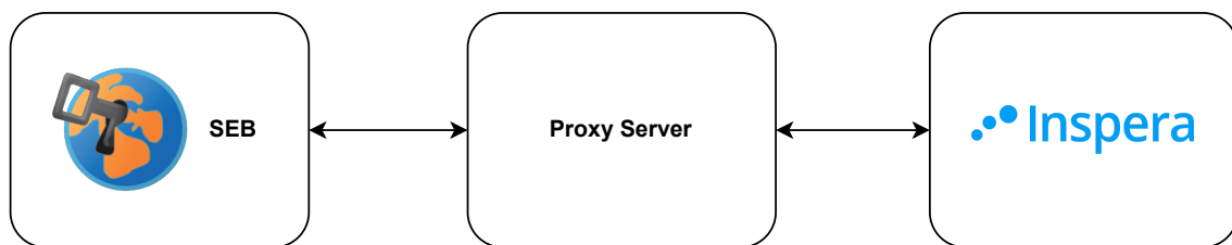
Figure 7.4: Flow between Safe Exam Browser and Inspira, where the Proxy Server works in a MITM manner, having access to all traffic sent between the two parties.
