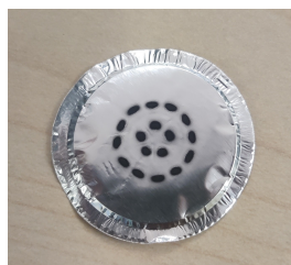
Figure 3.10: Aluminium foil with brake particles from the impactor (Stage 11)
