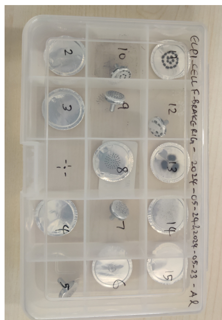
Figure 3.12: Al foils from all stages collected for SEM analysis
