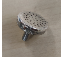
Figure 3.13: Aluminium foil mounted on a stud for SEM analysis
