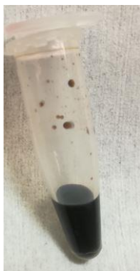
Figure 32: Photograph of Pt 3 Y sputtered onto [Emim] [OTf] for t = 3 \times 300 s.
