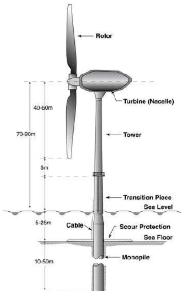
Figure 1: Wind turbine components (Source: Malhotra, 2011)
