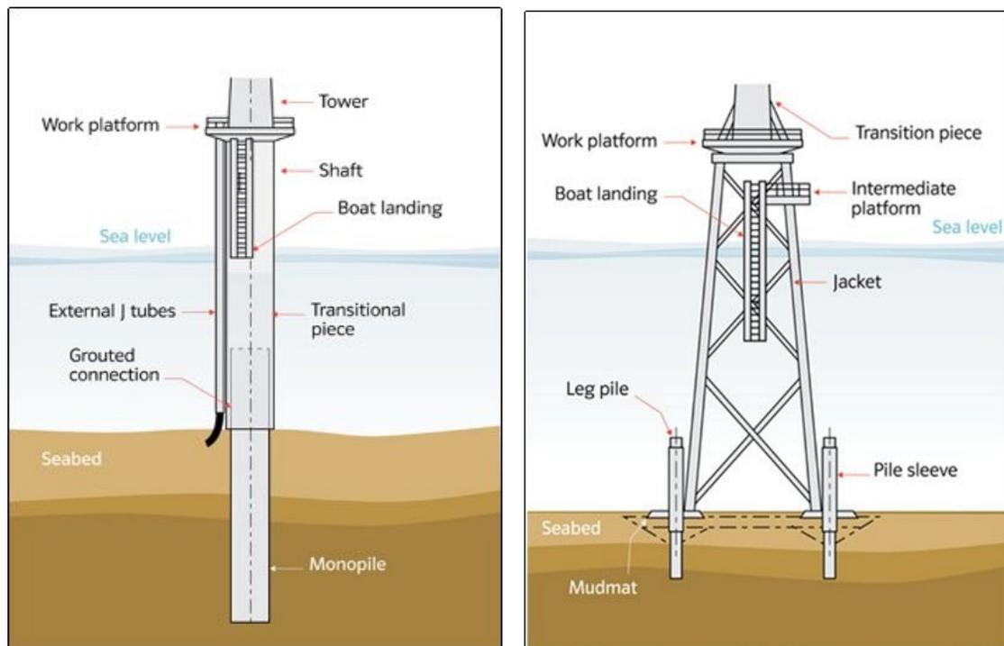
Figure 2: Monopile foundation (left) and Jacket foundation (right), (Source: 4coffshore 2013).
