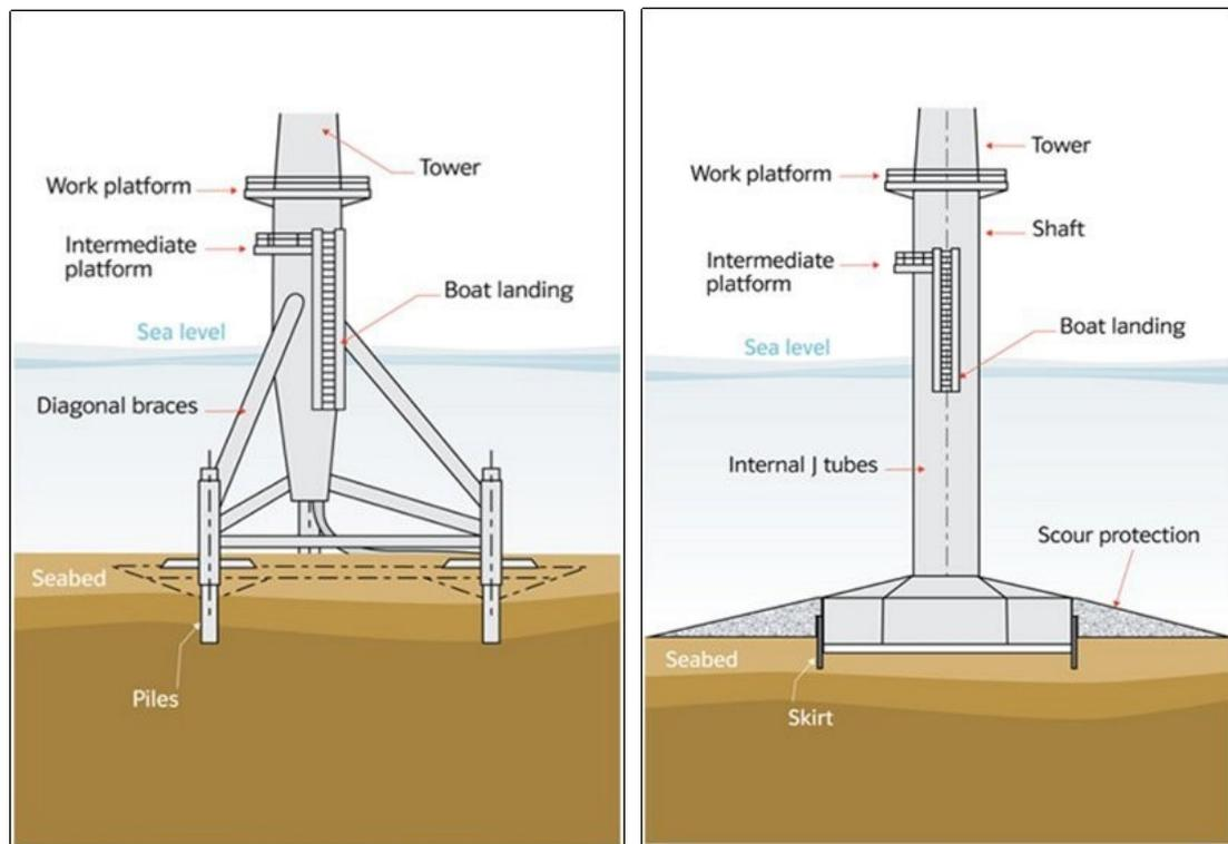
Figure 3: Tripod foundation (left) and Gravity foundation (right) (Source: 4coffshore 2013)
