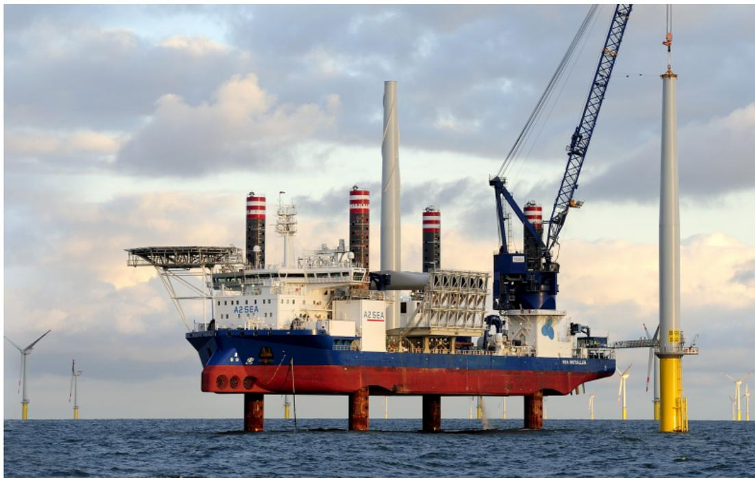
Figure 4: Jack-up rig/Jack-up vessel (Source: Offshorebiz 2016)
