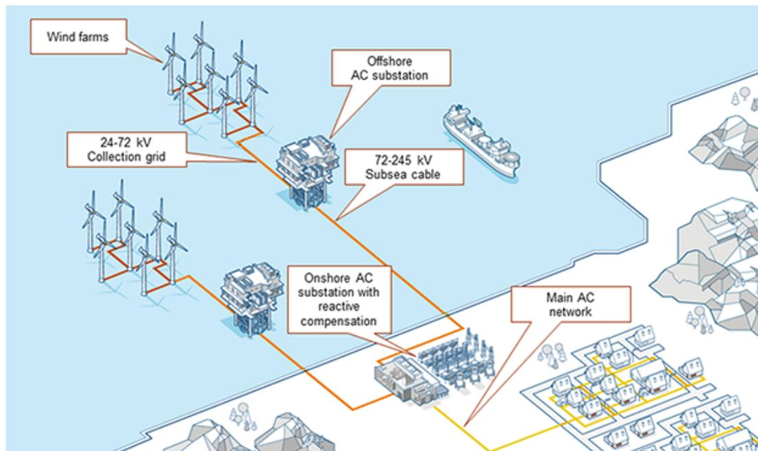
Figure 5: Offshore wind farm layout (Source: ABB)
