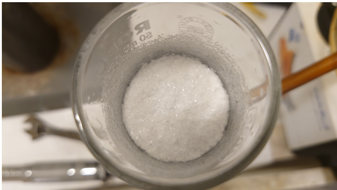
Figure 4.15: The resulting caprolactam after reaction using the Ru/10Sr-ZrO 2 catalyst, showing the ease of filtration of the caprolactam
