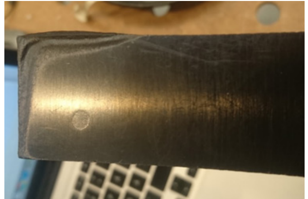
Figure 5.7 Deformation of pure PPS after 20 seconds
