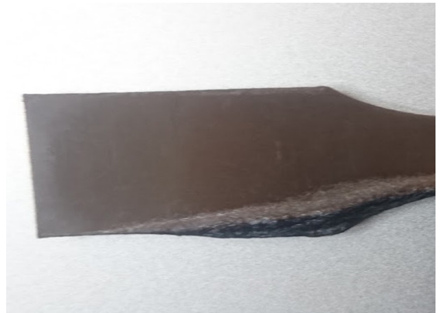
Figure 5.8 Deformation of 40% glass-fibre reinforced PPS; 20 seconds on the upper half of the piece and 30 on the lower
