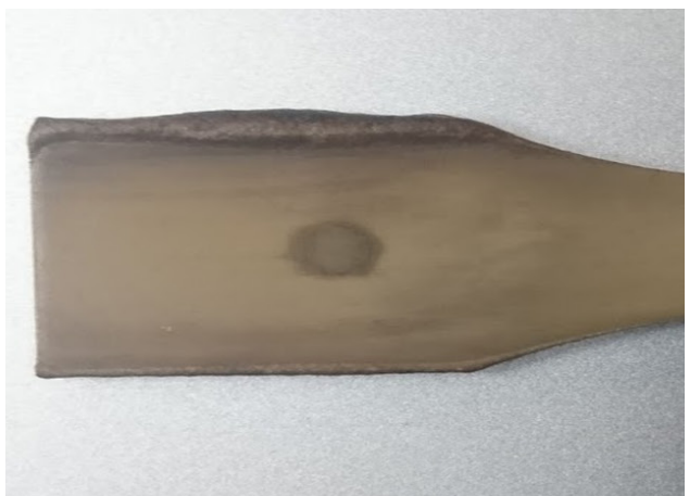
Figure 5.8 Deformation of PEEK; 30 seconds at the top of the image below, and 20 on the bottom of the image.
