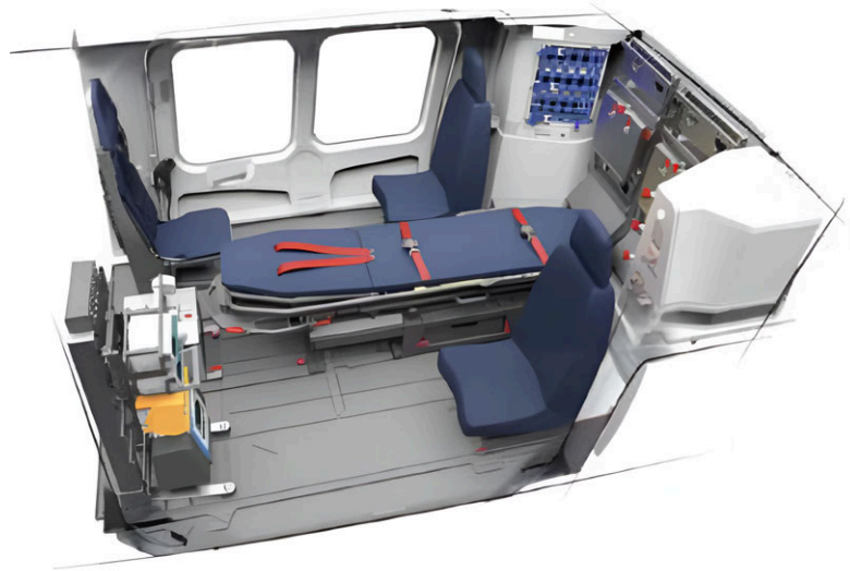
Figure 2.7: Cabin layout of Swedish ambulance helicopter Leonardo AW169 (Avincis, n.d.-b). Reprinted with permission.
