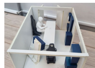
Figure 3.3: The 1:10 scale model, with 3D-printed equipment, seats and a sitting manikin.
