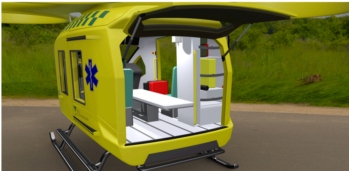
Figure 8.2: Back view of the interior, showing the rear entrance storage, stretcher and seats.
