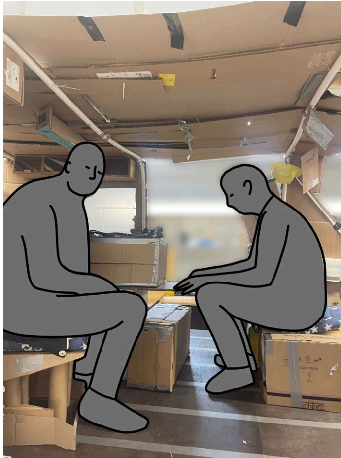
Figure 7.6: Participants evaluating the cabin space, seat and stretcher height as well as the seat-stretcher-configuration.
