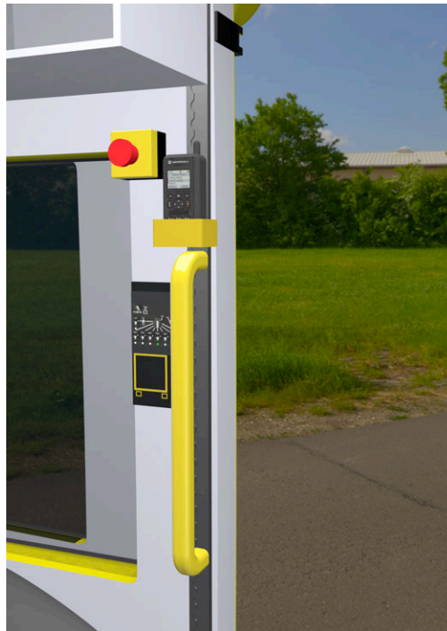
Figure 8.3: Radio communication device, stop button, handle and on the nurse's side of the UAM.
