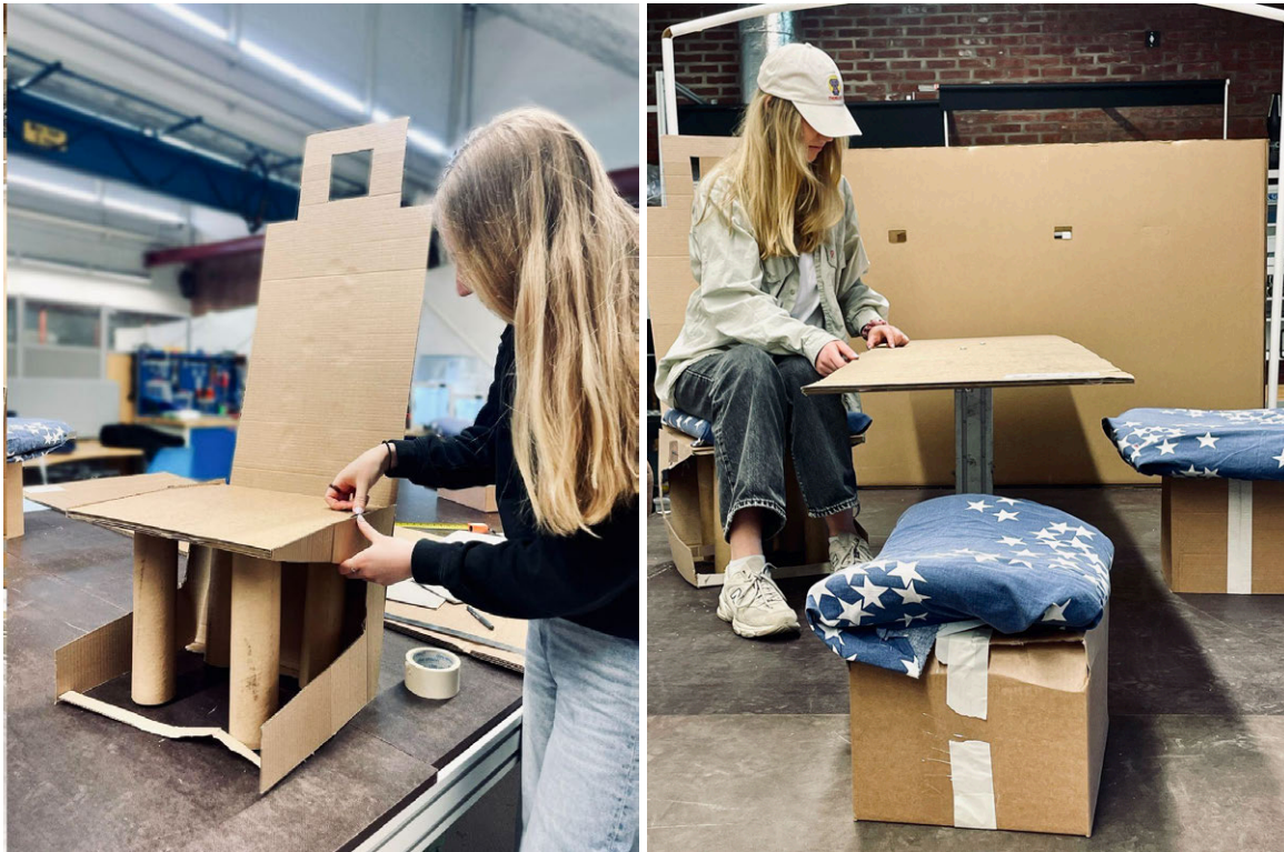
Figure 6.12: Building the seats and the stretcher and testing the seat-stretcher configuration in the full-scale.
