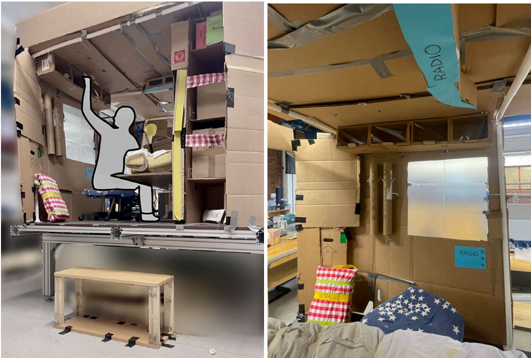
Figure 6.19: Own testing of the ceiling-storage, to ensure reachability of items inside. The tester is 168 cm tall.
