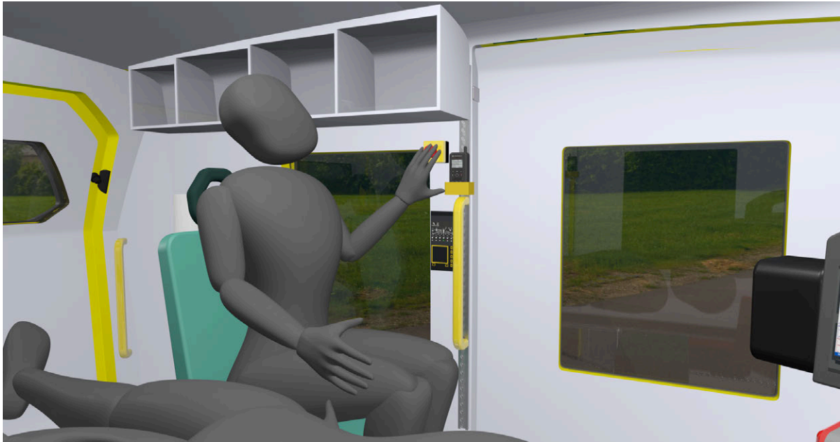
Figure 8.15: Nurse pushes the stop button on the wall next to the right-side entrance, to override the autonomous system, making the UAM top and hover in the air.
