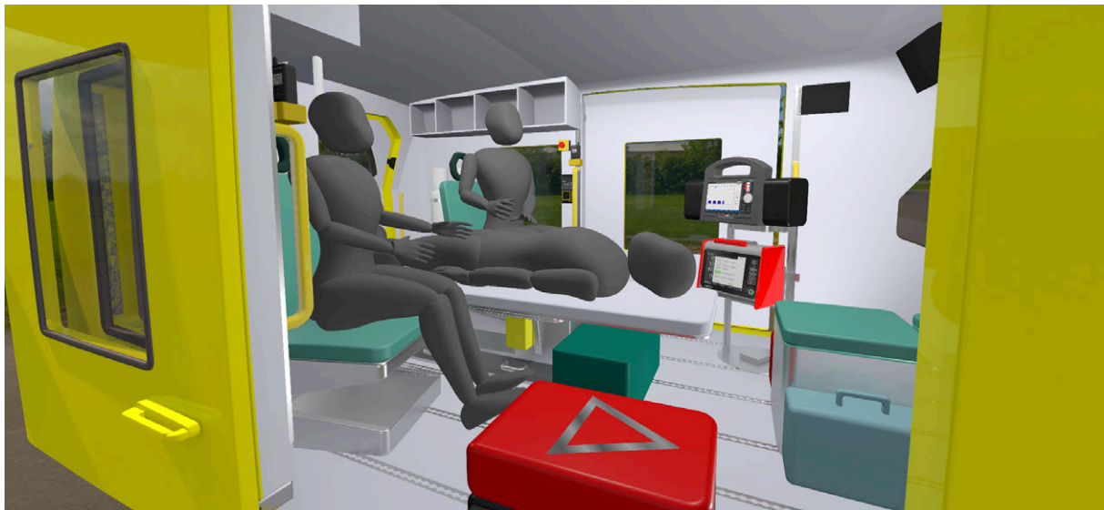
Figure 8.1: Side view of the interior, showing ceiling-storage, seat-stretcher configuration and monitoring devices rack.
