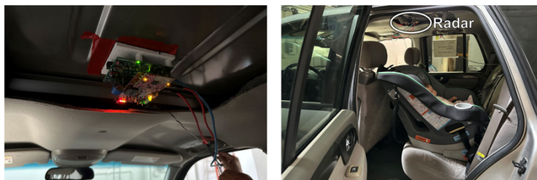
Figure 2.2: Radar mounted to the ceiling of the cabin for in-vehicle occupant classification, from [8].
