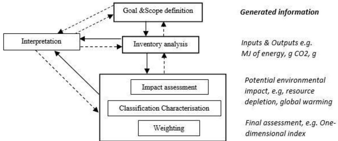
Figure 5: The LCA Procedure (Adapted from (Tillman, 2004) )
