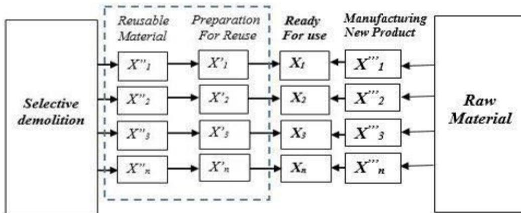
Figure 6: Selective demolition plan
