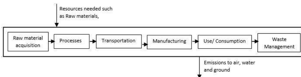
Figure 4: LCA model (Adapted from: (Tillman, 2004))
