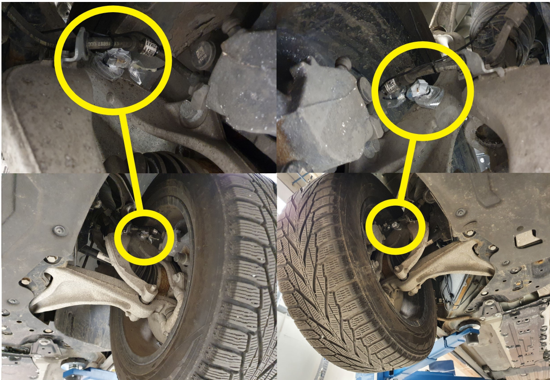
Figure 3.13: The two front three-axis accelerometers
