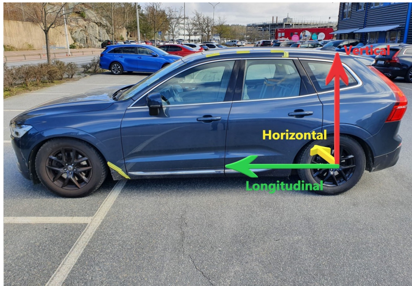
Figure 3.8: Vertical, Horizontal and Longitudinal axes along the car
