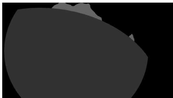
Figure 4.17: Segmented image of a degassing process. The dark gray ellipse on the bottom represents the lid of the ladle. The black area inside the boundaries is the obstructing slag.
