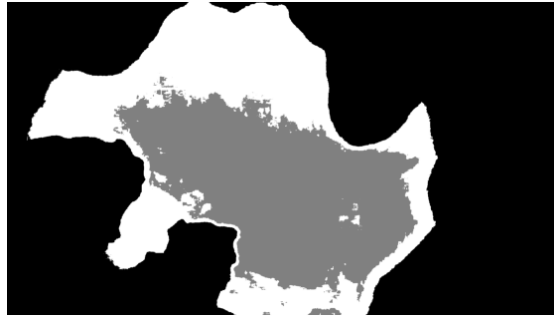
Figure 4.14: Segmenting an image of a degassing process into three classes using Gaussian Mixture Model. The black areas are the obstructions to the camera lens. The white areas are the wall of the ladle and some miss-classified fluid. The dark gray area is the moving fluid.
