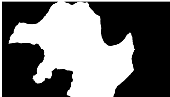
Figure 4.8: Binary filter extracted by using Otsu's threshold on an image of the degassing process. The black parts are obstructions to the camera vision. The white parts are the areas where the camera captures useful information.
