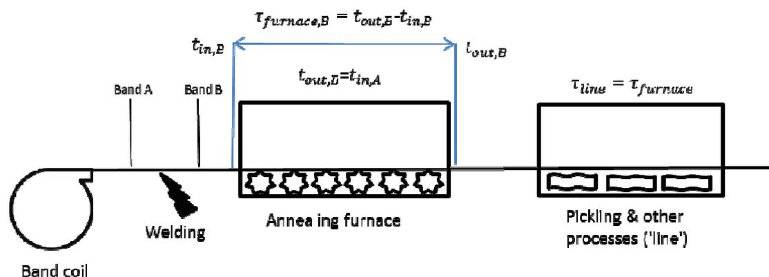
Figure 4.1 Residence times in the annealing and pickling line.
