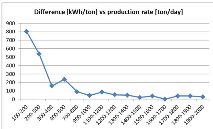
Figure C.4 Specific difference in-out of energy balance in relation to daily production rate.
