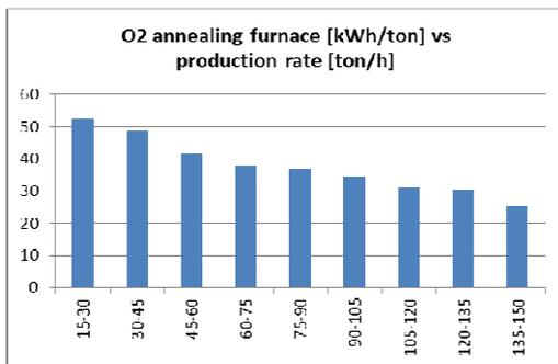
Figure 6.7 Specific oxygen energy consumption in annealing furnace in relation to production rate.
