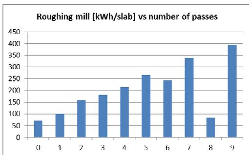
Figure 6.15 Roughing mill electricity consumption in relation to number of passes.
