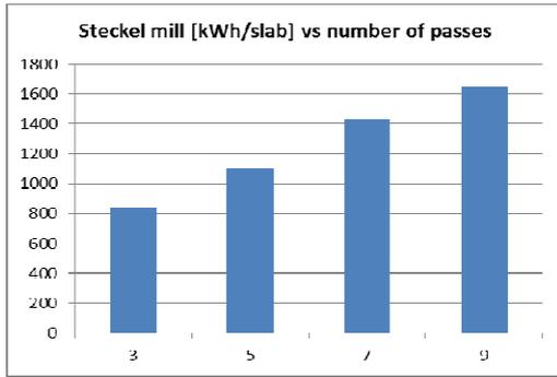
Figure 6.12 Steckel mill electricity consumption in relation to number of passes.
