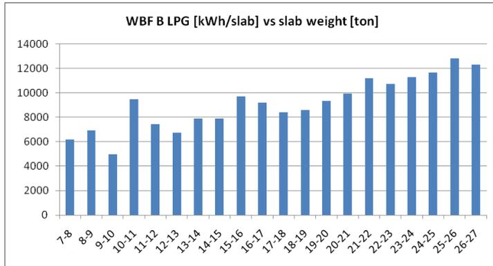
Figure 6.17 LPG consumption of WBF B in relation to slab weight.
