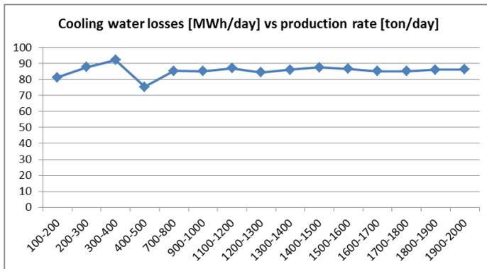
Figure C.1 Cooling water losses in relation to daily production rate.
