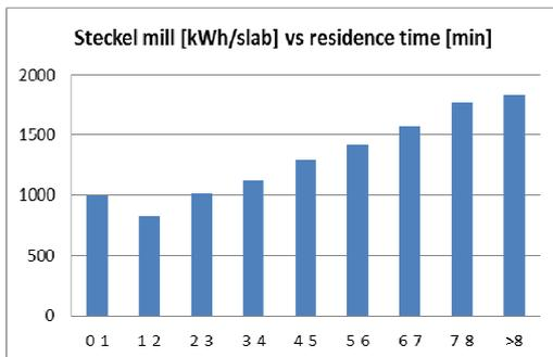
Figure 6.11 Steckel mill electricity consumption in relation to residence time.
