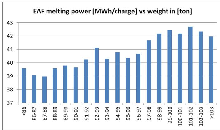
Figure 6.22 EAF melting power consumption in relation to charge weight.
