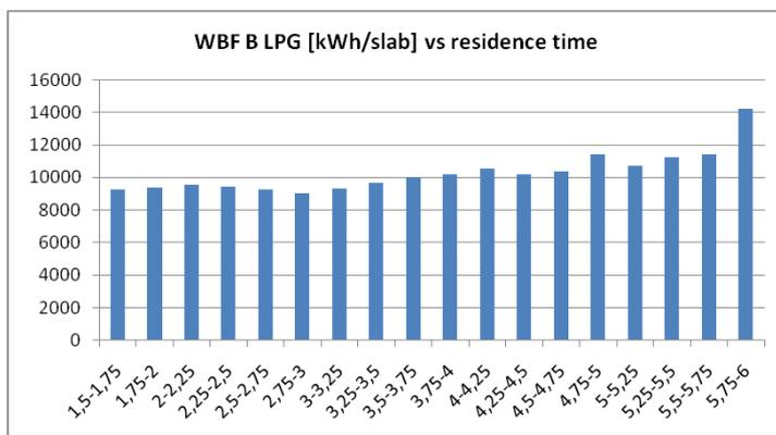
Figure 6.19 LPG consumption of WBF B in relation to residence time.
