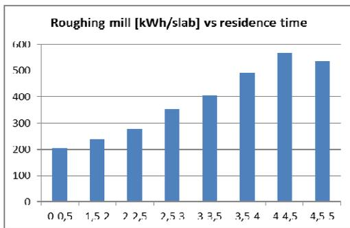
Figure 6.14 Roughing mill electricity consumption in relation to residence time.
