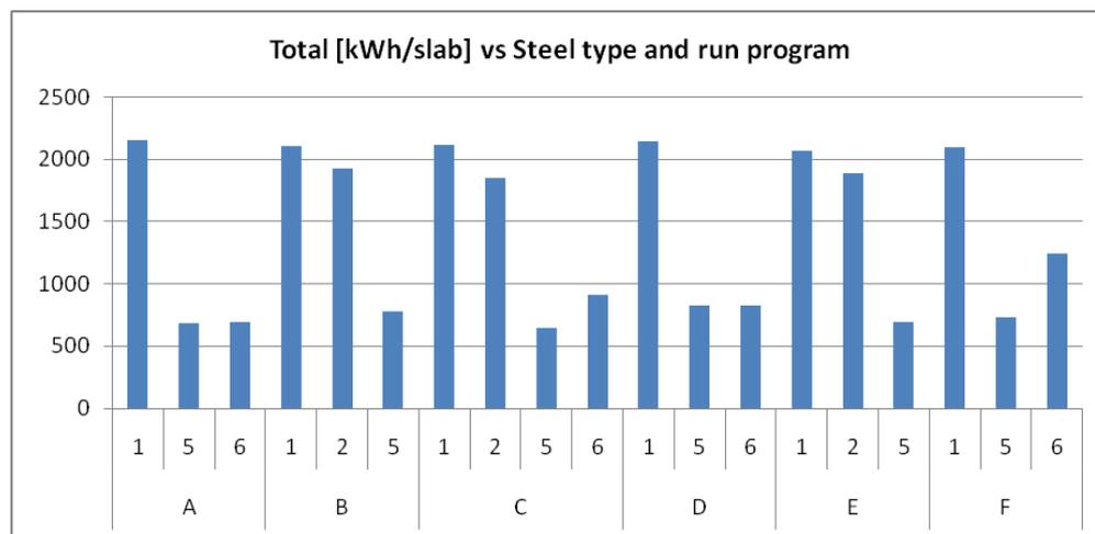
Figure 6.8 Total electricity consumption in relation to steel type and 'run program'.
