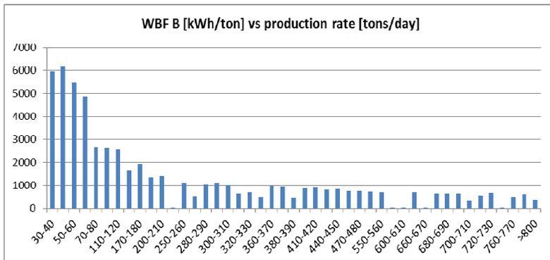
Figure 4.3 Daily specific energy consumption for WBF B for different daily production rates.
