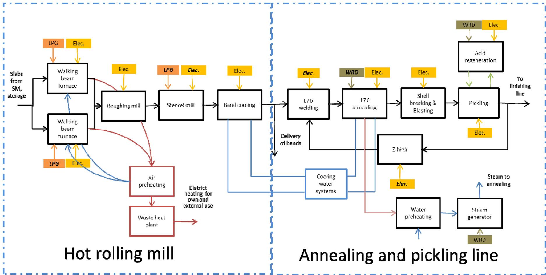
Figure 2.2 Simplified process flowsheet for the hot rolling mill and the annealing and pickling line.
