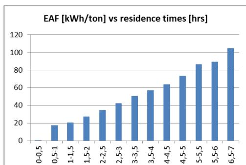
Figure F.2 Specific electricity consumption for auxiliaries and scrap preheating in the EAF in relation to residence time.
