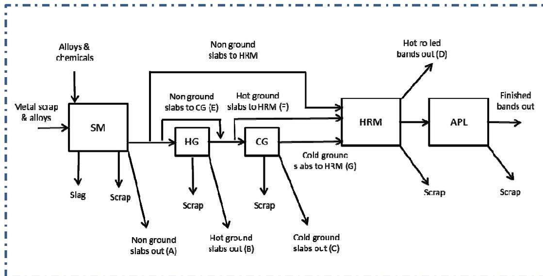
Figure 3.1 Flow of products in the production process.
