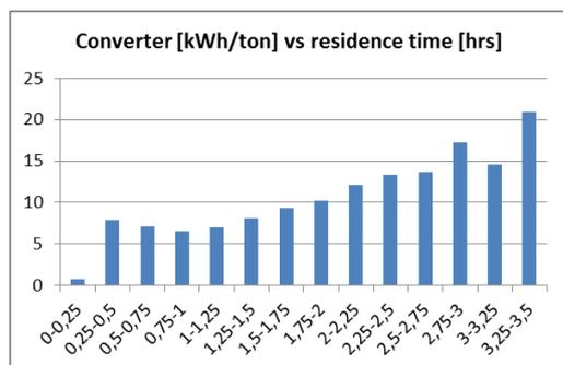
Figure F.3 Specific electricity consumption for the converter in relation to residence time.
