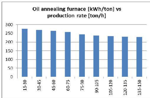
Figure 6.6 Specific WRD oil consumption in annealing furnace in relation to production rate.
