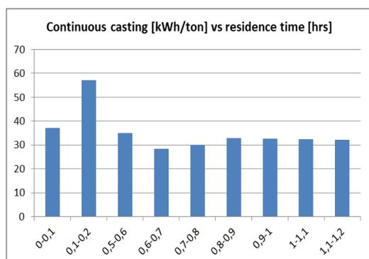
Figure F.5 Specific electricity consumption for the continuous casting in relation to residence time.
