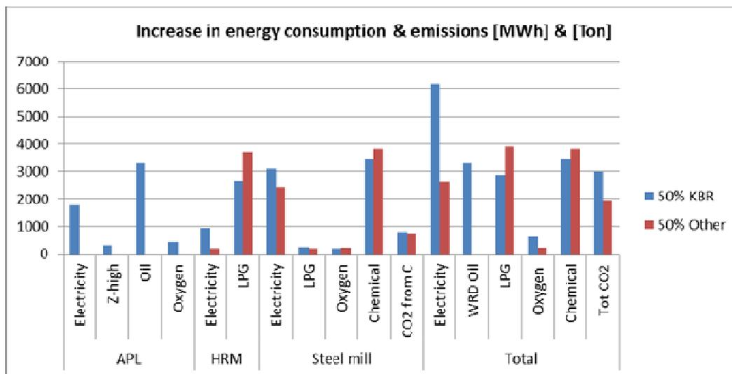
Figure 8.1 Absolute increase in energy consumption for production scenarios.
