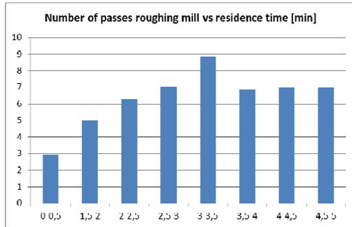
Figure 6.16 Roughing mill number of passes in relation to residence times.
