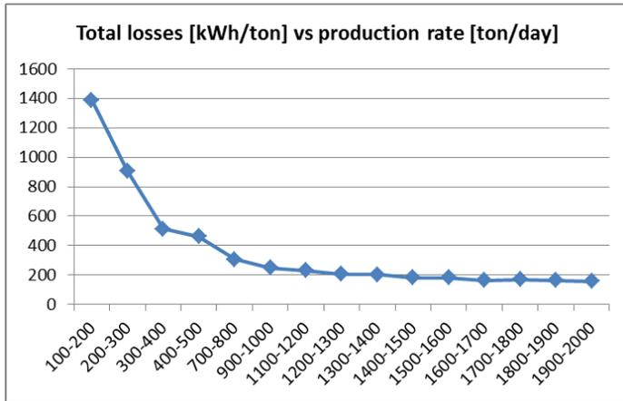
Figure C.3 Total specific losses in relation to daily production rate.
