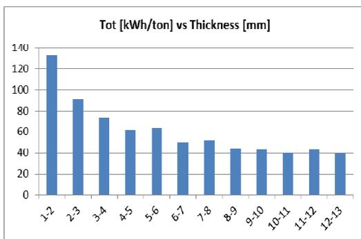
Figure 6.4 Total specific electricity consumption in relation to thickness.
