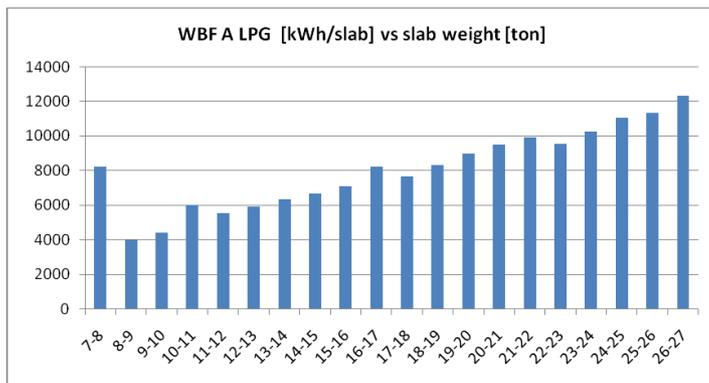
Figure 6.18 LPG consumption of WBF A in relation to slab weight.
