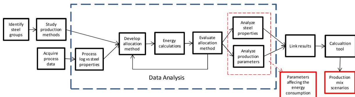
Figure 1.1 Flowchart of analysis procedure.
