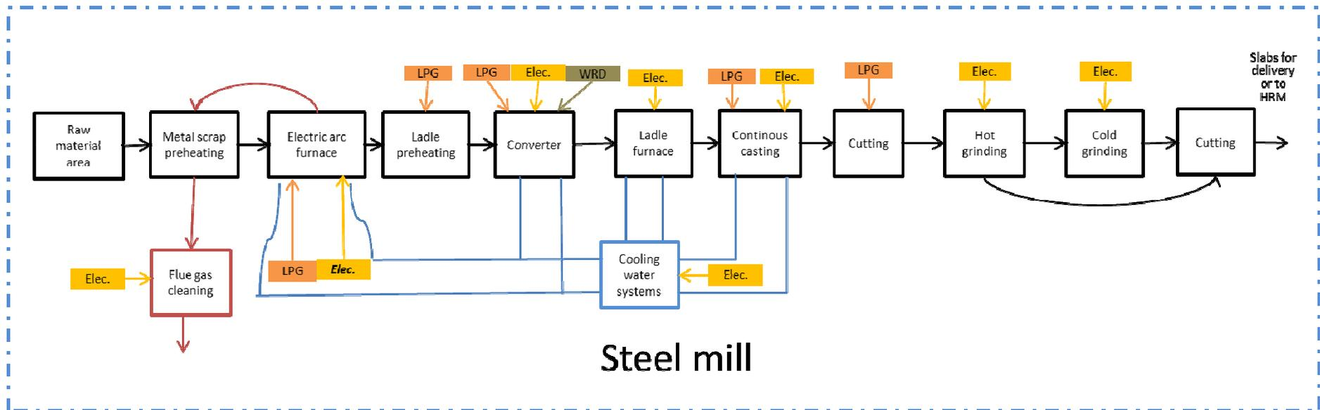
Figure 2.1 Simplified process flowsheet for the steel mill.
