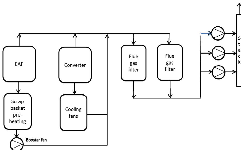
Figure 4.5 Schematic of the flue gas system in the steel mill.
