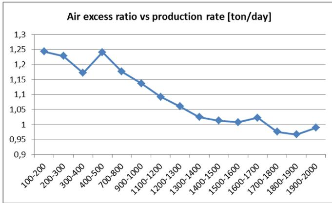
Figure C.5 Air excess ratio in relation to daily production rate.
