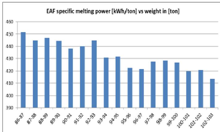
Figure 6.23 EAF specific melting power consumption in relation to charge weight.
