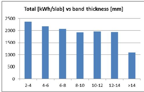
Figure 6.10 Total electricity consumption in relation to band thickness.
