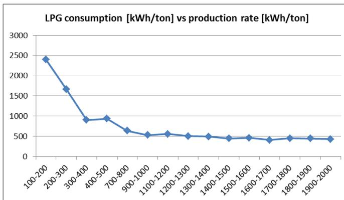
Figure C.2 Specific LPG consumption in relation to daily production rate.
