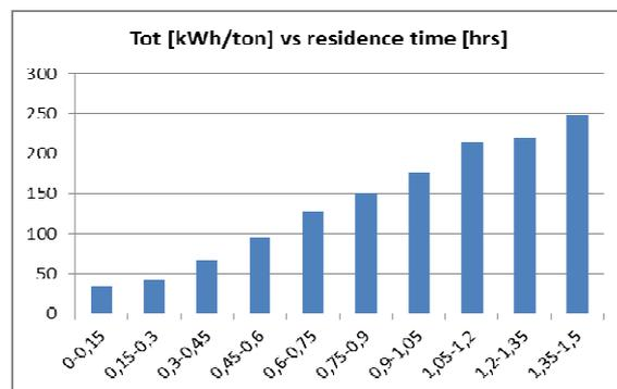
Figure 6.1 Total specific electricity consumption in relation to residence time.
