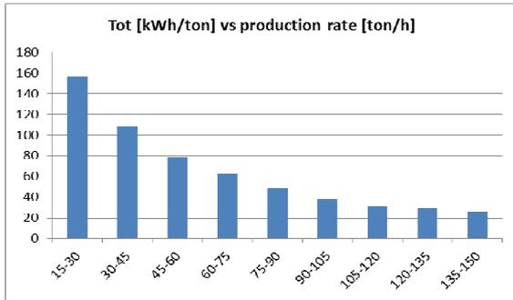
Figure 6.2 Total specific electricity consumption in relation to production rate.
