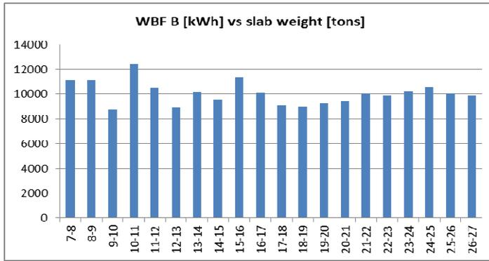
Figure 4.2 LPG consumption for WBF B, based on residence time only.
