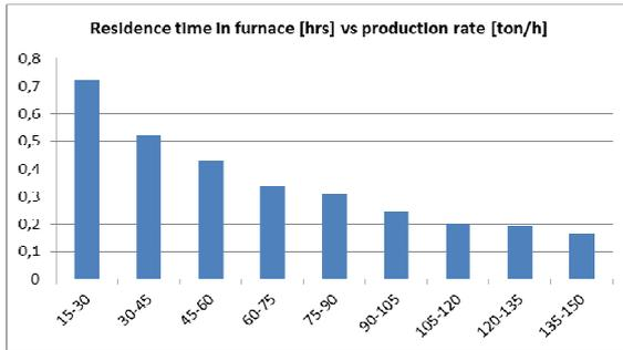
Figure 6.3 Residence time in furnace in relation to production rate.
