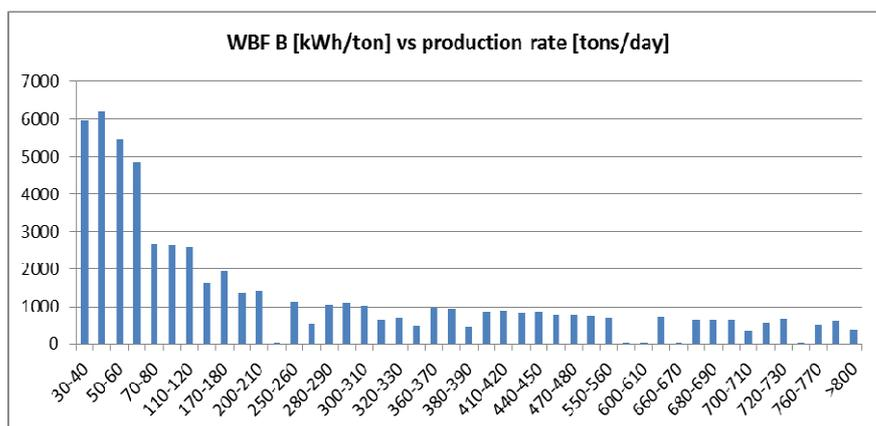
Figure 6.20 Daily specific energy consumption of WBF B in relation to daily production rate.
