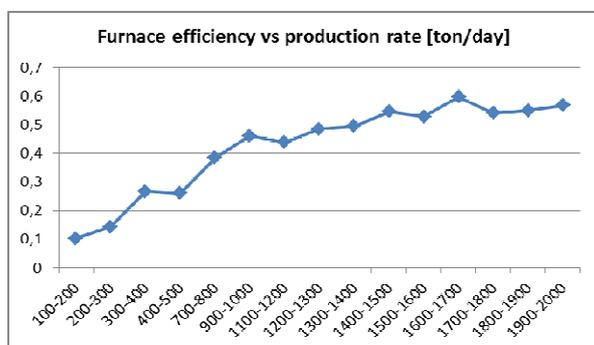
Figure 6.21 Furnace efficiency in relation to daily production rate.
