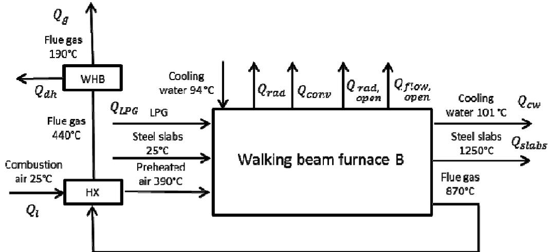
*Figure 4.4* Heat balance for WBF B.
