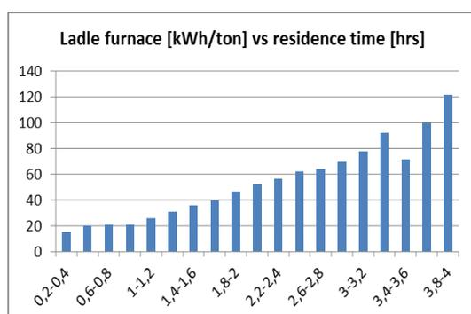
Figure F.4 Specific electricity consumption for the ladle furnace in relation to residence time.
