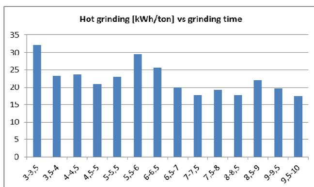
Figure F.1 Specific electricity consumption of the hot grinding in relation to grinding time.
