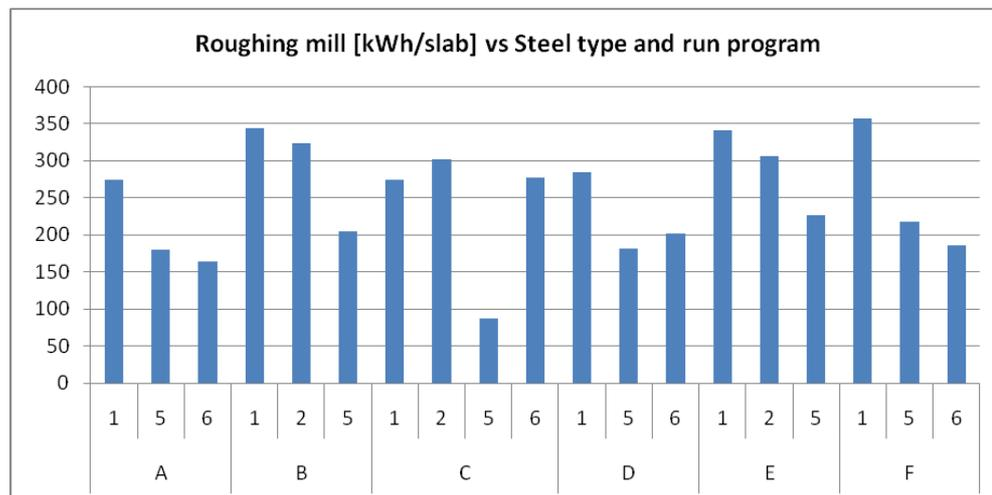
Figure 6.9 Roughing mill electricity consumption in relation to steel type and 'run program'.
