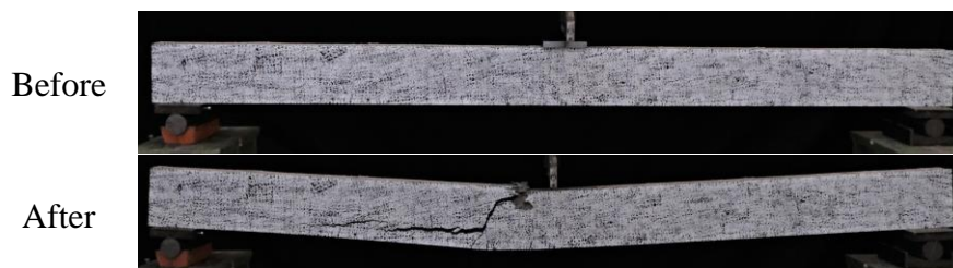
Figure K.3 Images of beam B-06 before and after static loading.
