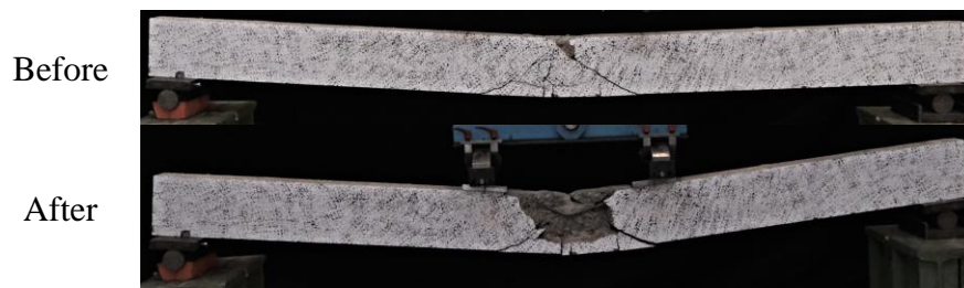
Figure L.5 Images of beam B-15 before and after static loading.
