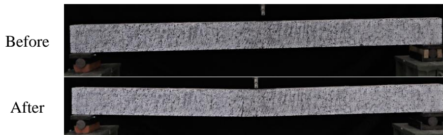
Figure K.1 Images of beam B-02 before and after static loading.
