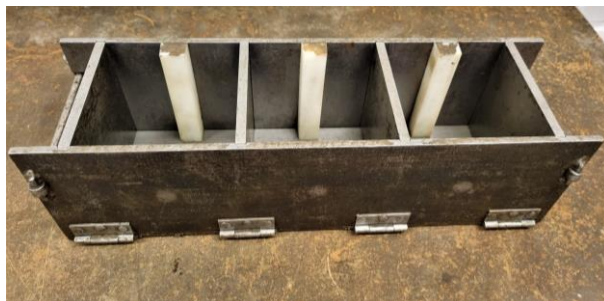
Figure 6.4 An illustration of the casting of cubes used for wedge splitting tests.
