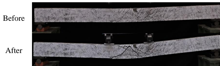
Figure L.6 Images of beam B-16 before and after static loading.
