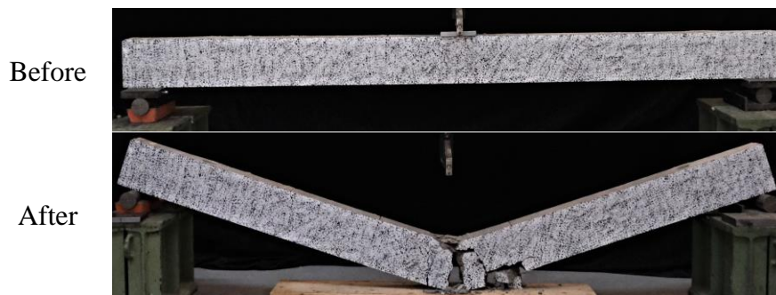
Figure K.2 Images of beam B-04 before and after static loading.
