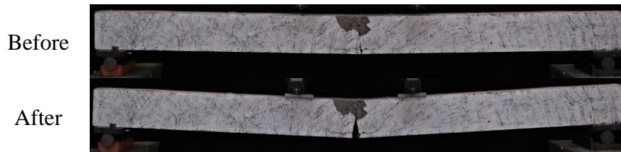
Figure L.1 Images of beam B-08 before and after static loading.
