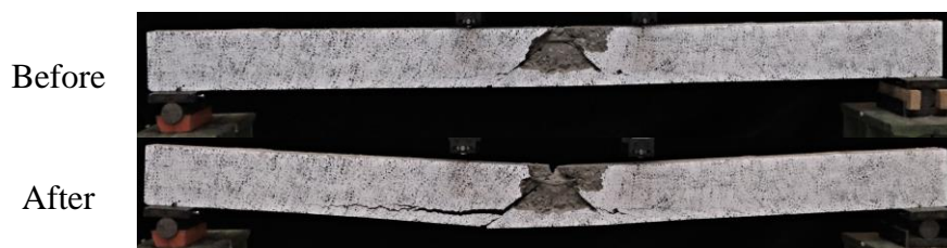
Figure L.4 Images of beam B-13 before and after static loading.
