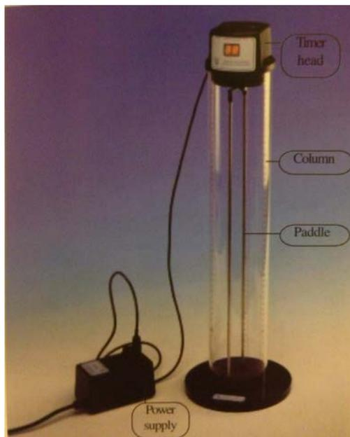
Fig 3.1 The Triton-WRc settling apparatus
