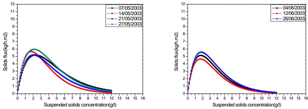
Fig 5.5 Relation between solids flux and concentration of sludge (2003)
