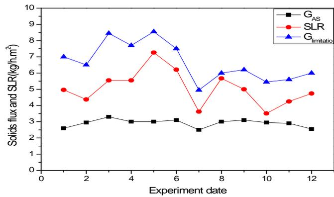
Fig 5.10 Relation of applied solids flux value, limitation solids flux value and solids loading rate
