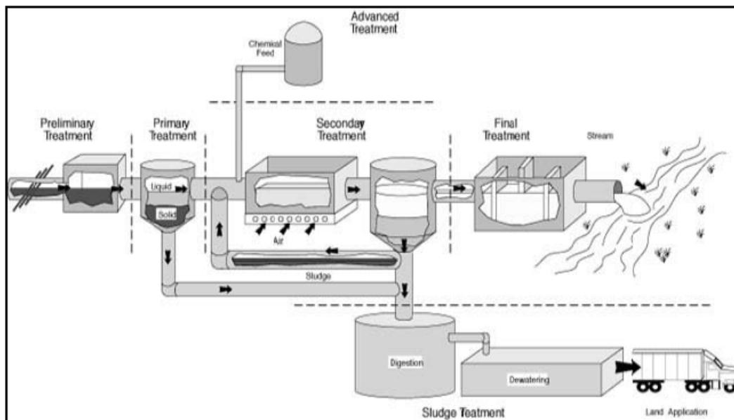
Figure 2. Schematic drawing of a typical wastewater treatment plant. [1]
