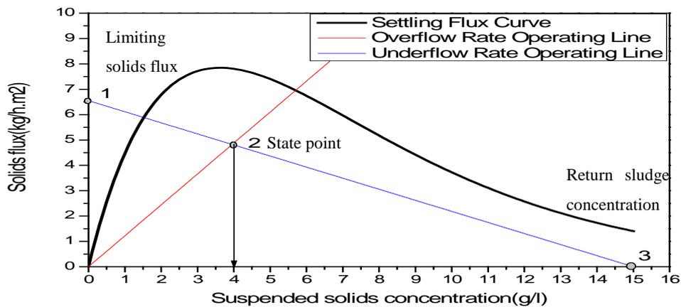
Fig 2.3 State point analysis in a secondary settler
