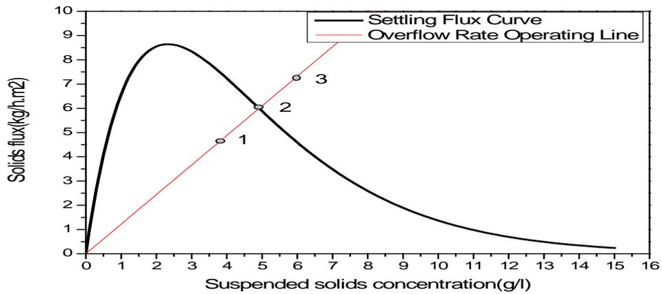
Fig 2.4 State point analysis for assessing clarifier operating
