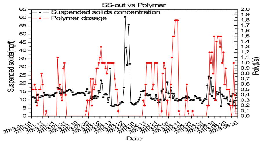
Fig 5.15 relation between Suspended solids concentration and polymer dosing
