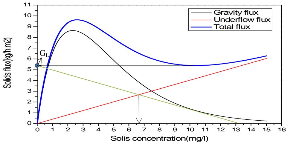
Fig 2.2 Definition sketch for the analysis of settling data using solids flux method.
