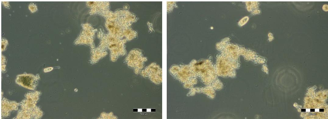
Fig 7.6 Microscopic pictures of the flocs at 10x and 20x, respectively (14/6).
