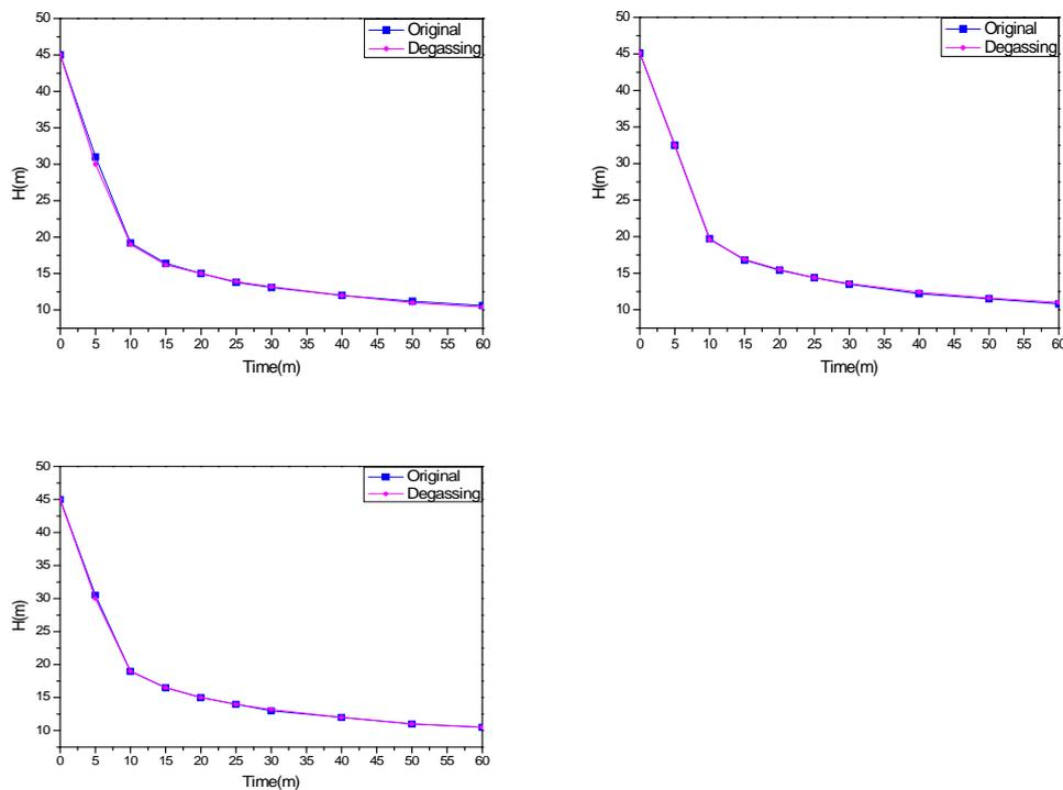
Figure 6.1 Comparison of the zone settling velocity between non degassed sample and degassed sample
