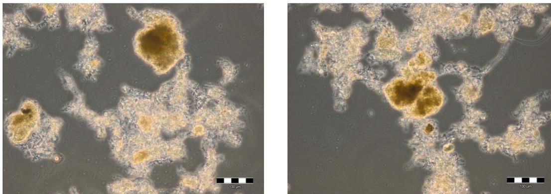
Fig 6.2 Microscopic pictures of the non-degassed and degassed flocs, respectively
