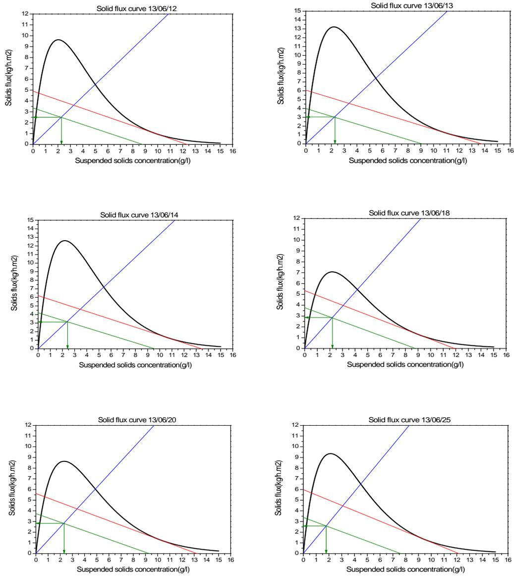
Fig 5.9 Solids flux curves with determination of the state point.
