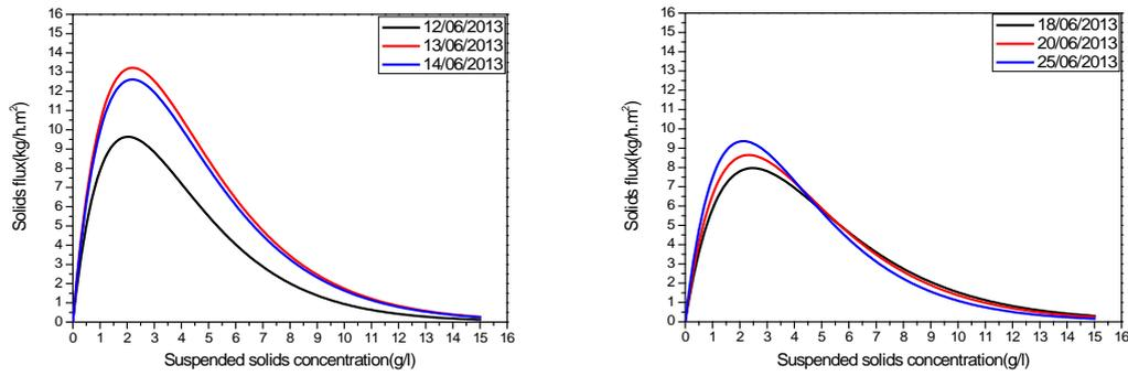
Fig5.3 Relation between solids flux and concentration of sludge(2013)
