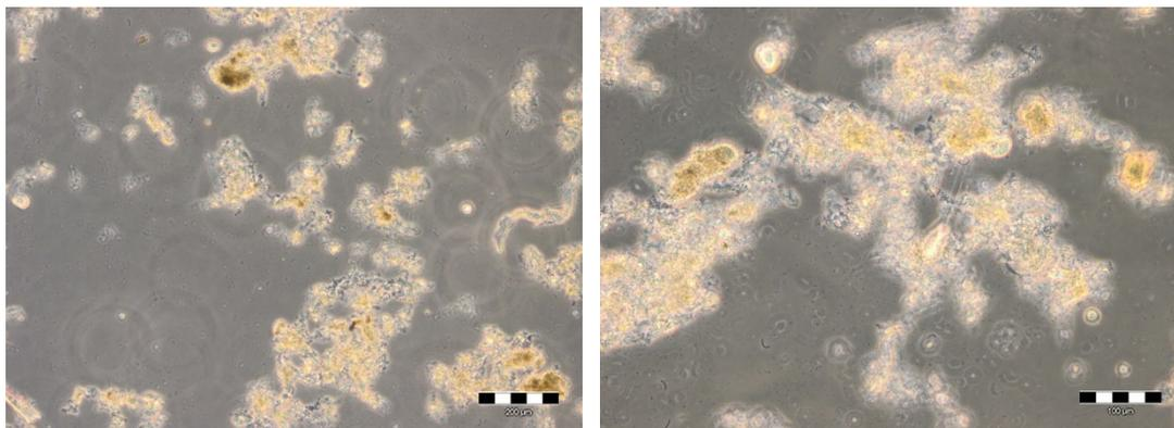
Fig 7.2 Microscopic pictures of the flocs at 10x and 20x, respectively (21/5).
