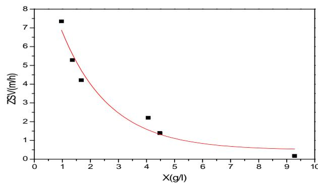
Fig2.11 Example curve of the Vesilind model
