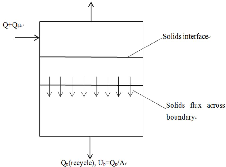
Fig 2.1 Definition sketch for a settling basin operating at steady state [4]
