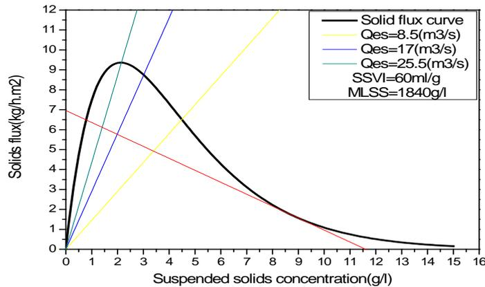
Fig 5.8 Compared with different inflow in secondary settler
