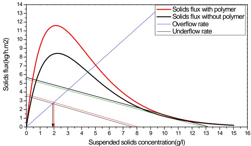
Fig 5.13 Solids flux curves with determination of the state point in the polymer test
