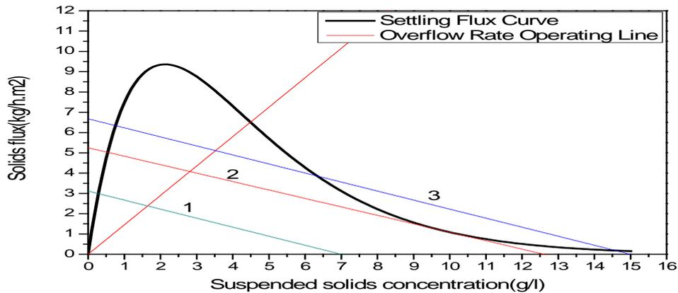
Fig 2.5 State point analysis for assessing thickened operating
