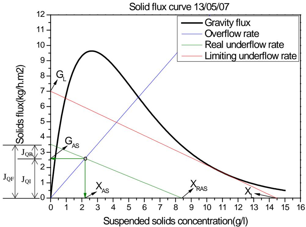
Fig 2.6 Definitions of the settling flux curve and state point analysis of SST operation
