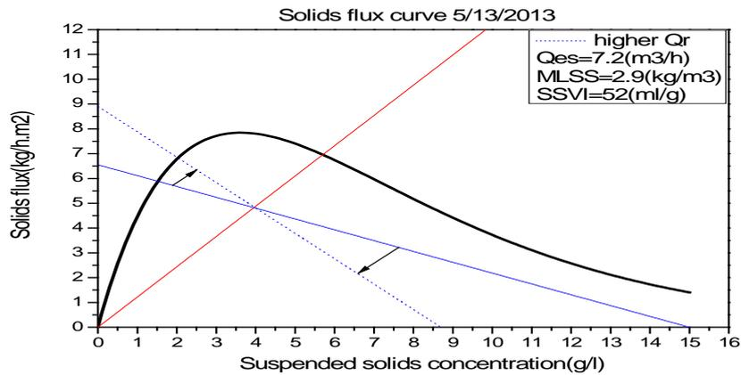
Fig 2.9 Effect on return sludge flow
