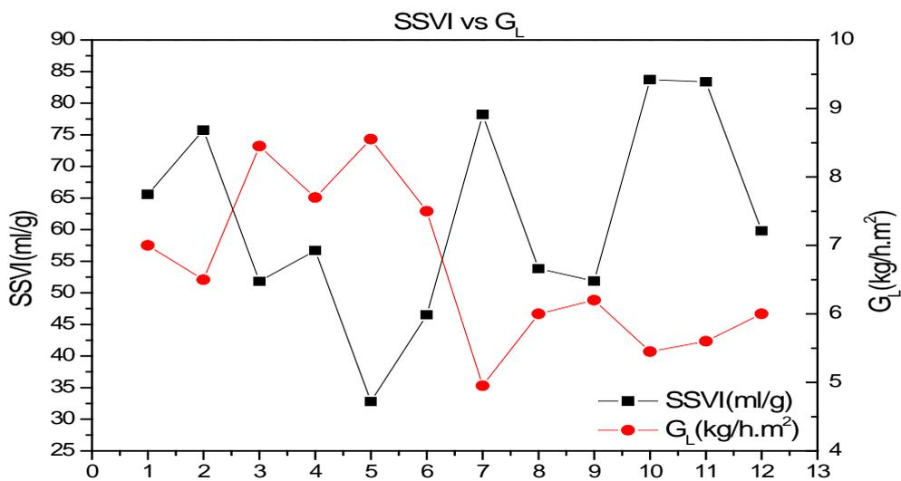
Fig6.12 Relation of SSVI and limitation solids flux
