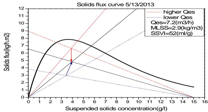
Fig 2.7 Effect on influent flow into secondary settler
