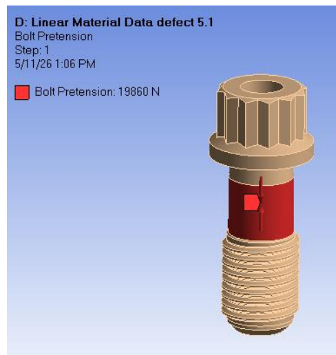
Figure 3.3. Pretension loading procedure in ANSYS.
