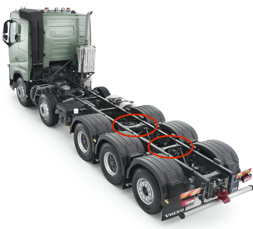
Figure 4.1: Location of bogie cross member on the chassis, from [52]
