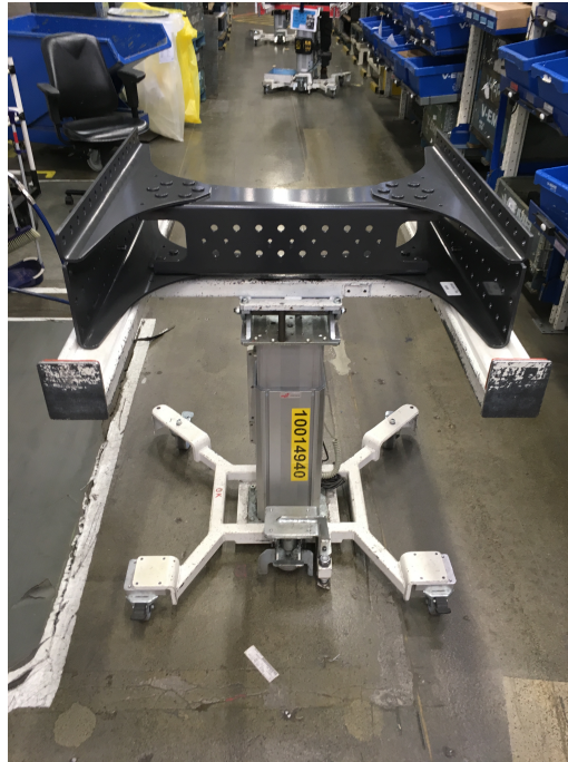
Figure 4.4: Bogie cross member on the trolley used in subassembly
