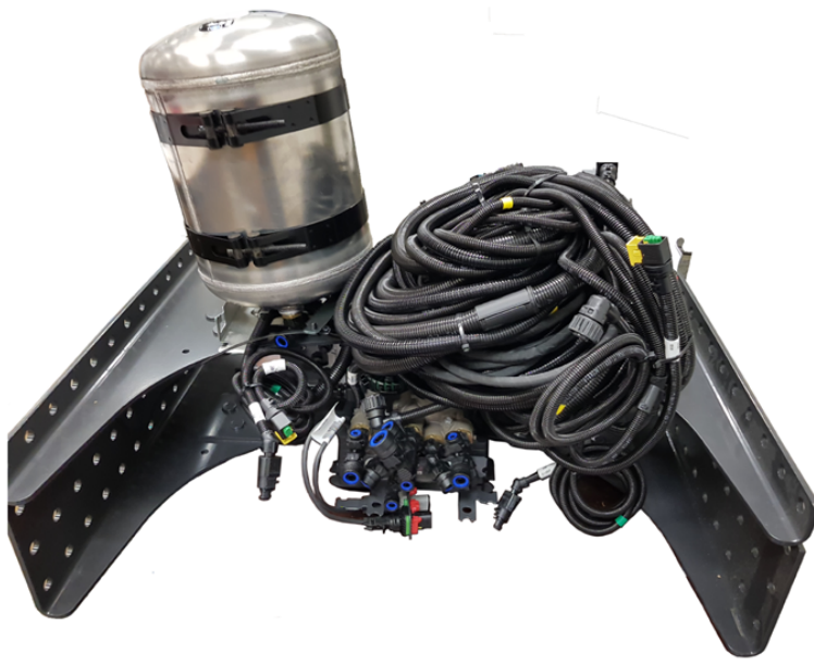
Figure 4.2: Fully equipped bogie cross member, positioned upside down
