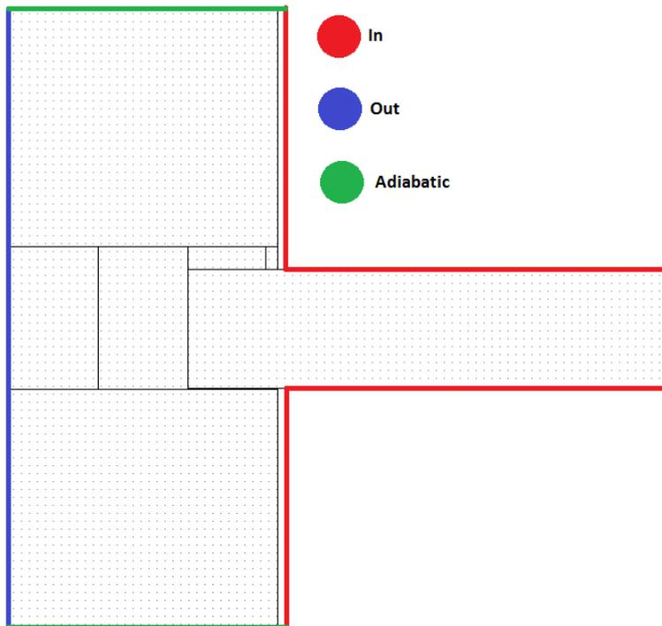
Figure 4, Basic geometry with boundary conditions
