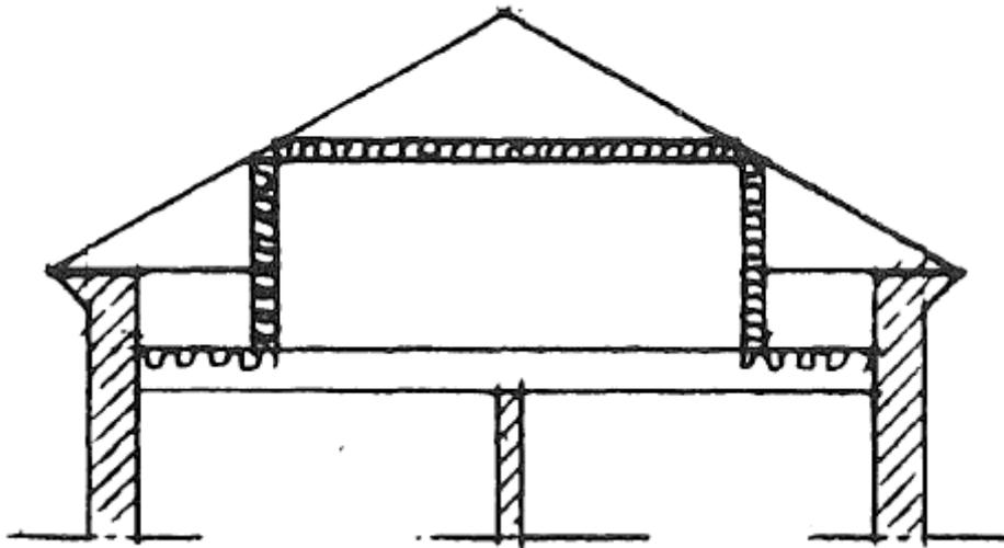
Figure 4.2 Section of an alternative to attic apartments (Bjerking, 1974).
