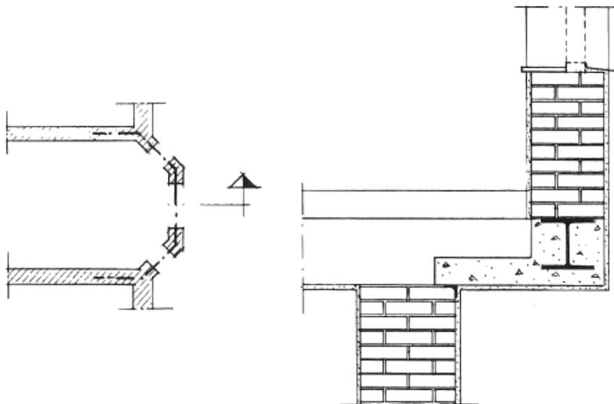
Figure 3.10 Bay window construction (Bjerking, 1974).
