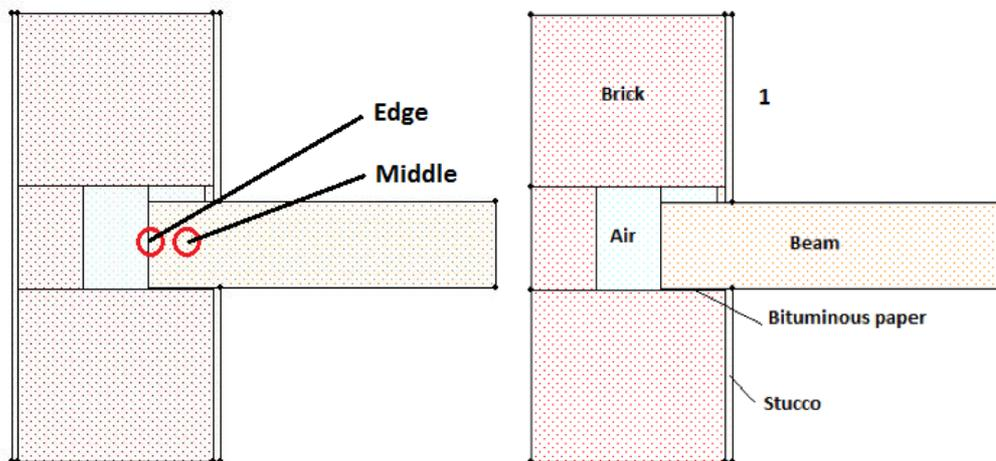
Figure 6.3 Left: Original beam box and unmodified model used for simulations of the support of the slab in the wall, including measuring points. Right: Material assigned in the model.
