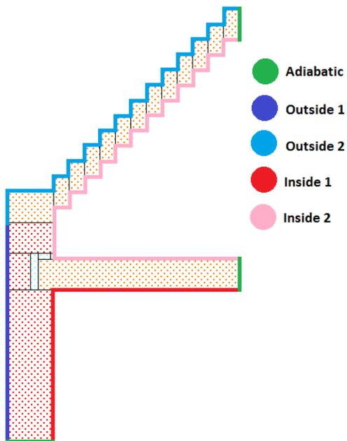
Figure 4, basic geometry with boundary conditions
