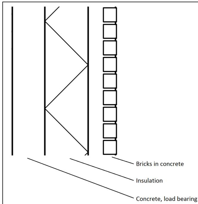
Figure 4.3 Section of a new sandwich element with remounted bricks (Strängbetong, 2016).
