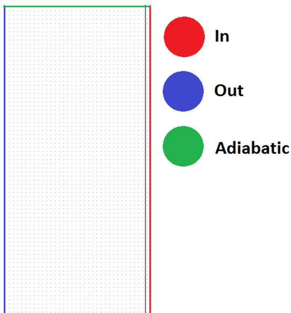
Figure 3, basic geometry with boundary conditions
