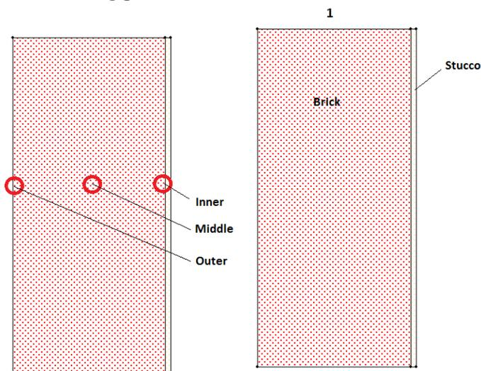
Figure 6.2 Left: Original wall and unmodified model used for simulations of the wall, including measuring points. Right: Material assigned in the model.
