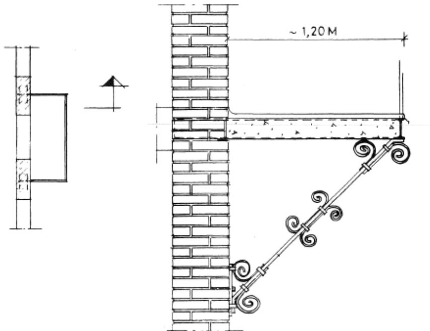
Figure 3.9 Balcony construction (Bjerking, 1974).
