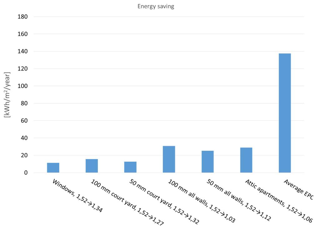
Figure 7.2 Diagram with energy savings due to U-value reduction from renovations and average EPC.
