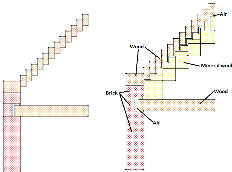
Figure 6.4 Left: Original roof-wall connection and unmodified model used for simulations of the connection wall – roof. Right: Insulated connection and material assigned in the model.
