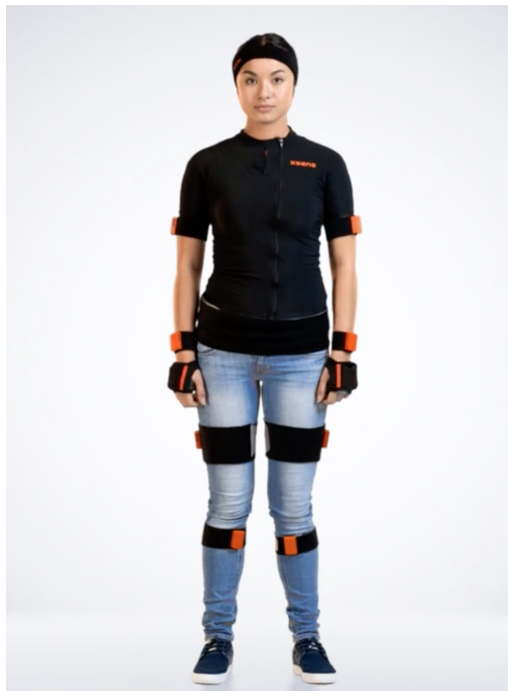
Figure 4.12: Image of a Xsens sensor placement on the test person (Source: Xsens.com)
