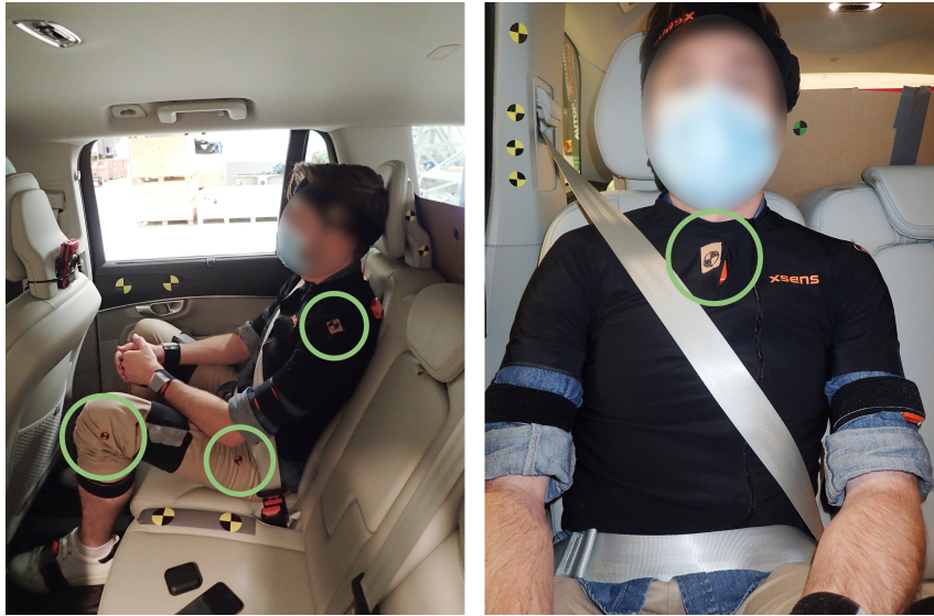
Figure 4.11: The stickers placed on the test persons used in the photo analysis
