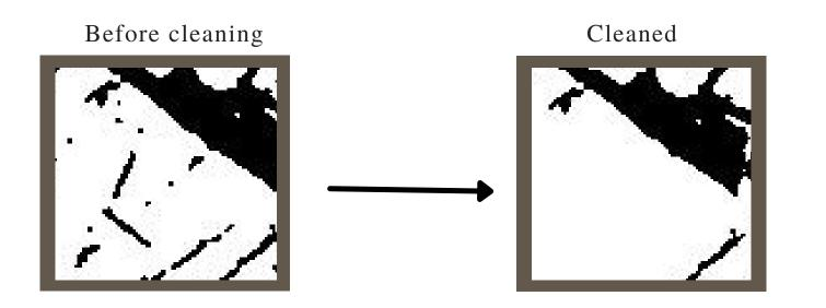
After the binary matrix is cleaned, it is possible to calculate the pores radius in each layer, by assuming each pore is a circle. The probability (frequency) of the pore dimensions are analyzed and related to the mass transport efficiency of the gas diffusion layer.
