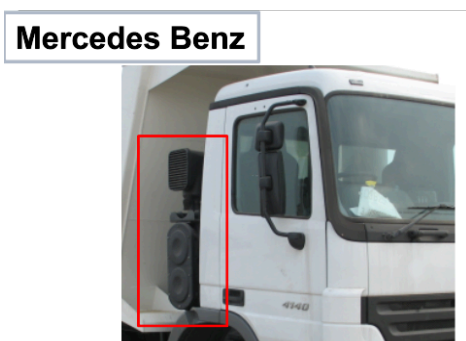
Figure 9: Dual air cleaner behind cab of Mercedes Benz truck. Internal Volvo Group presentation material, no longer publicly available.
