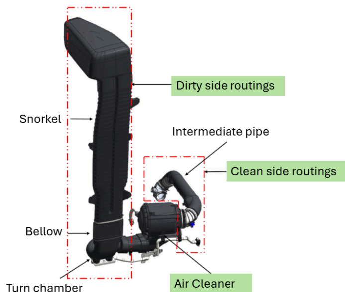
Figure 2: Picture of the air intake system. Source: Internal document.
