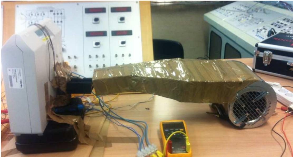
Fig. 6.28 Forced air cooling experimental set-up
