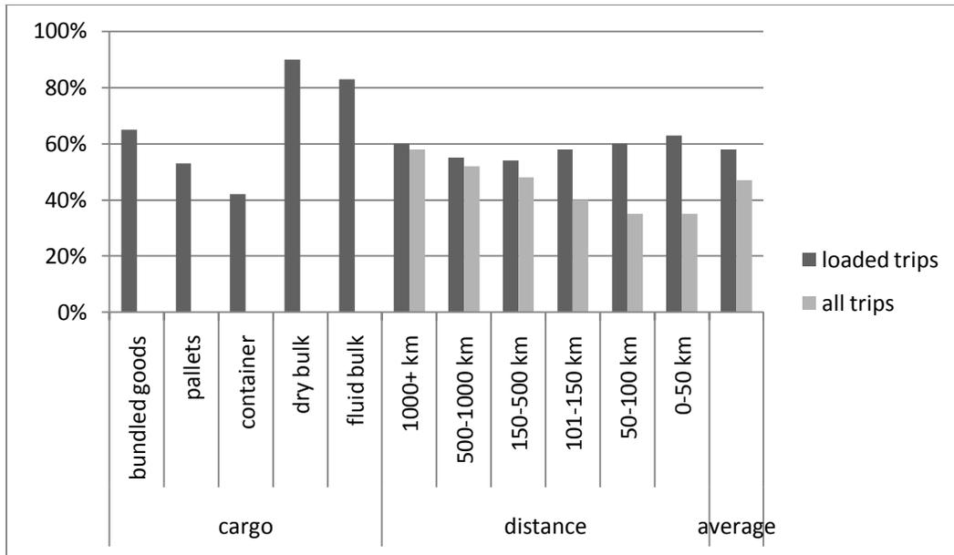
Figure 8, Load and utilization factors in Germany based on ton-km. note: loaded trips do not include empty return trip (den Boer, Brouwer, Schroten, & van Essen, 2009).
