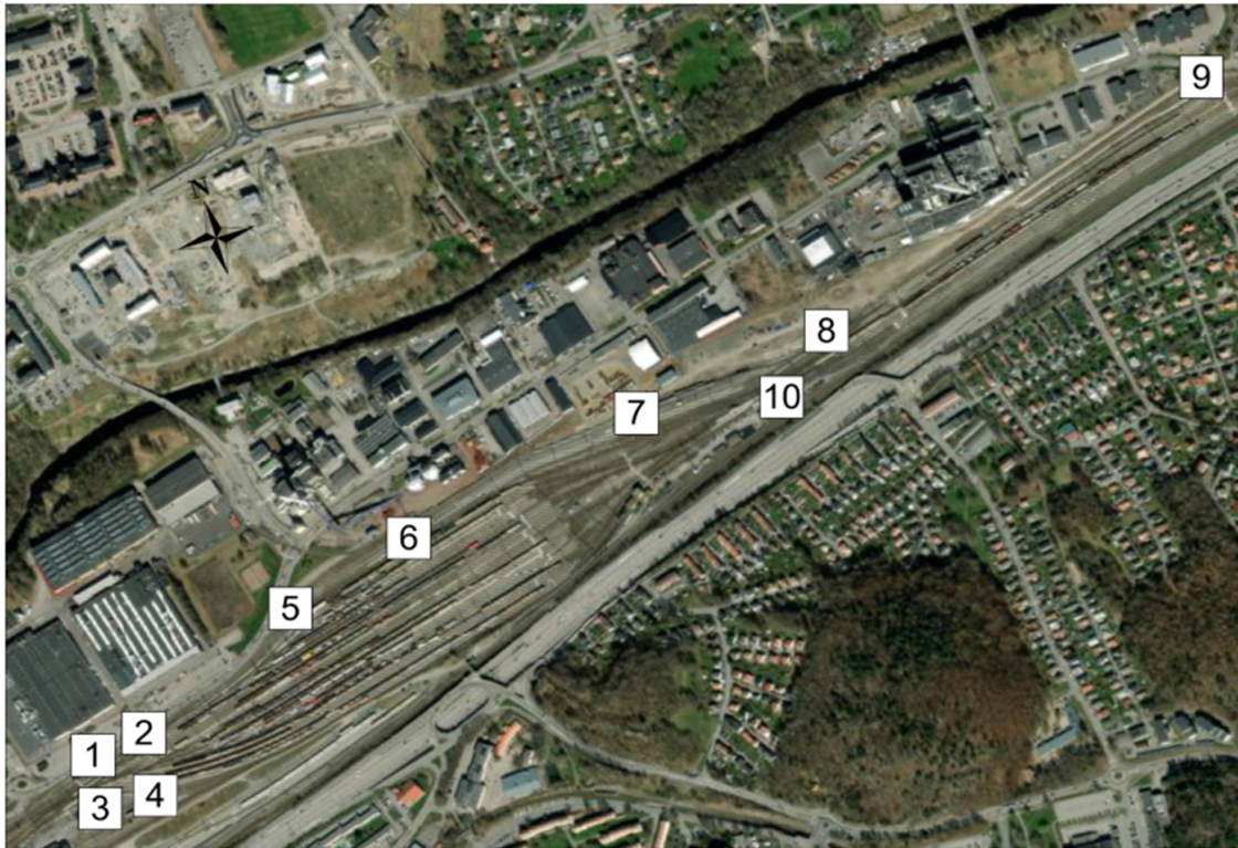
Figure 3.9: Placement of bellow hose measurements. From Trafikverket, [28].
