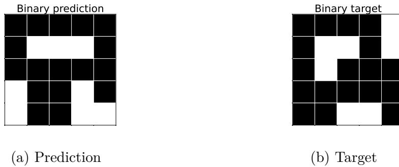
Figure 2.3: The binary prediction of a U-Net model (left) after a threshold has been applied to its output \mathcal{P} and its respective target mask (right). White pixels are classified as defects ( c = 1 ) and black pixels are classified as background ( c = 0 ). On a pixel basis there are 3 TP, 4 FN, 5 FP and 13 TN predictions. But if instead once considers defect contours, there are 2 TP, 1 FP and 1 FN.
