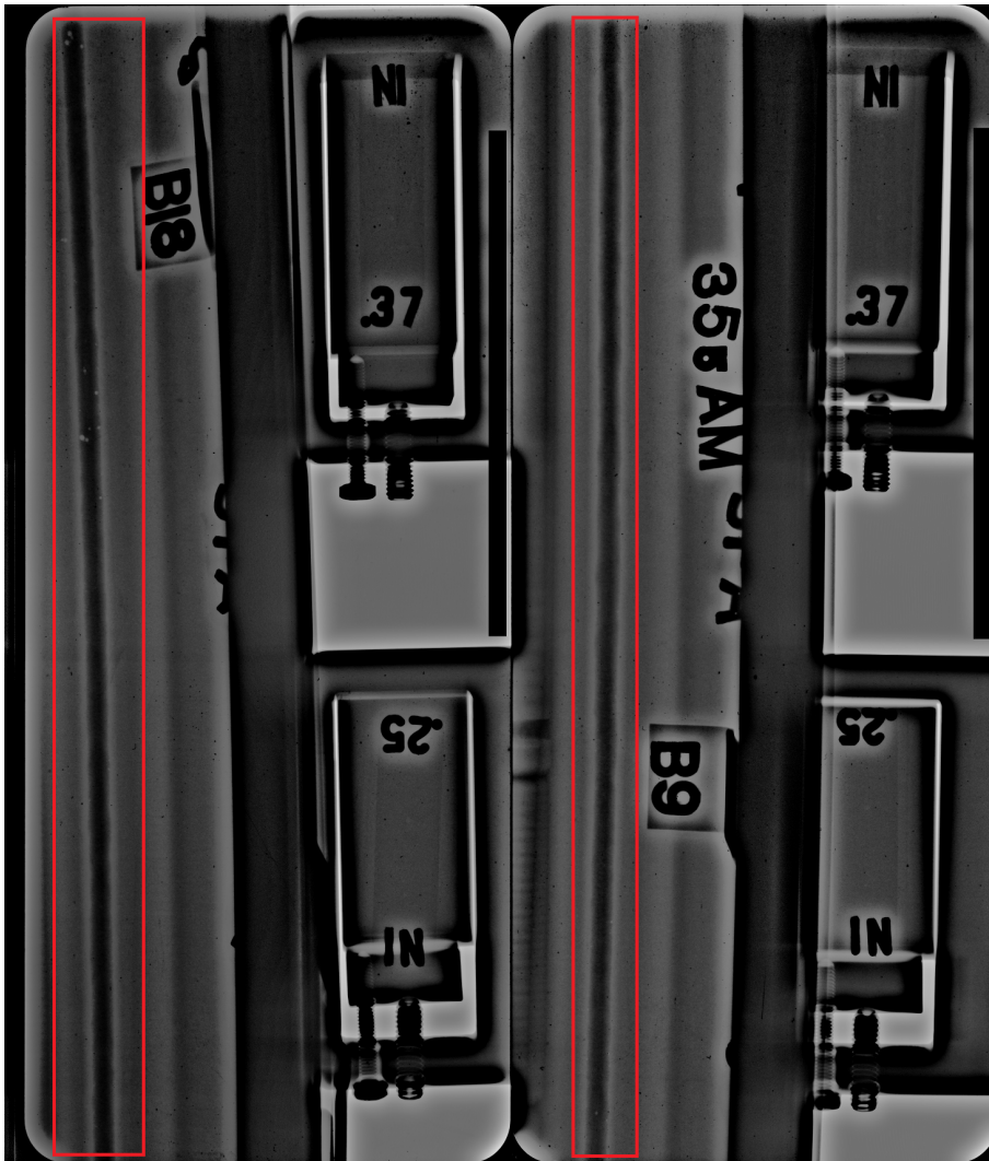
Figure 3.1: Full 5861 \times 6840 X-ray image taken of a weld segment. A 512 \times 512 sliding window traverses the full images and extracts image crops that are fed to the U-Net model. The weld regions are highlighted in the red bounding boxes. Small white speckles along the welds correspond to pores, indicative of defects that can potentially fail a component.
