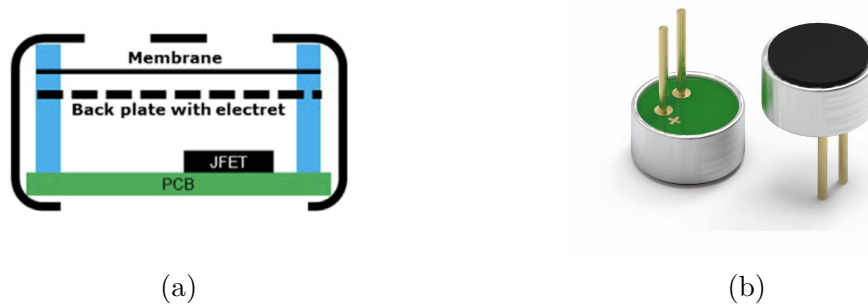
Figure 2.1: Cross-sectional sketch of ECM (a) and a real model – type LF-M6027-O from Ariose Electronics (b). Adopted from [45], [46].
