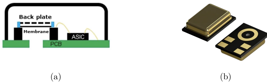
Figure 2.2: Cross-sectional sketch of MEMS (a) and a real model – type IMP23ABSU from STMicroelectronics (b). Adopted from [45], [49].
