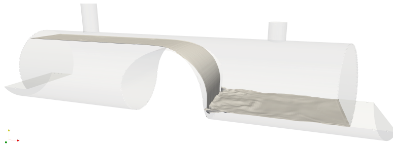
(a) Water level corresponding to a vertical blockage of 50% of the cross-sectional area
