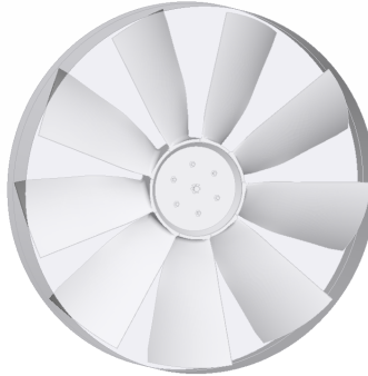
Figure 3.2: The fan blades with the interfaces for the rotating region.
