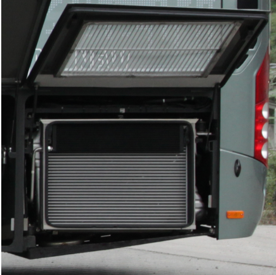
Figure 2.1: The cooling package, the oilcooler and CAC are visible in the bus and the radiator is behind the CAC. Image courtesy by Volvo Bus.
