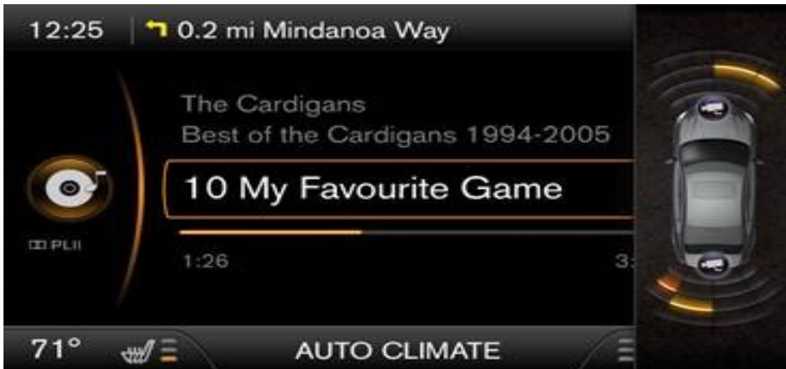
Figure 1.2: An image of HMI display from a Volvo car’s dash board. The right part of the image describes obstacles in the range using ultrasonic sensors mounted around the vehicle. The picture depicts the range of the sensors and displays positions of the obstacles. The golden brown and red coloured space around the car picture signifies a obstacle in that range.
