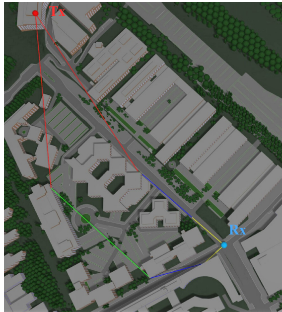
Figure 5.2: A couple of rays with multiple interactions traced between transmitter in red on top of a building and receiver in blue placed at the streets of Kista, Stockholm.
