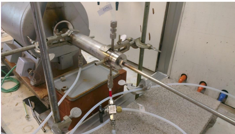
Picture 3 shows how the gases are connected, air on the top, the connection with the red strap is the argon and propylene inlet, the last one is the nitrogen.
