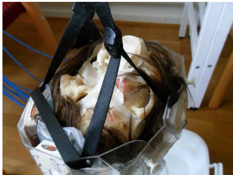
Figure 3.9: Cranium with wig placed in the MWH for measurements of the impact from hair.
