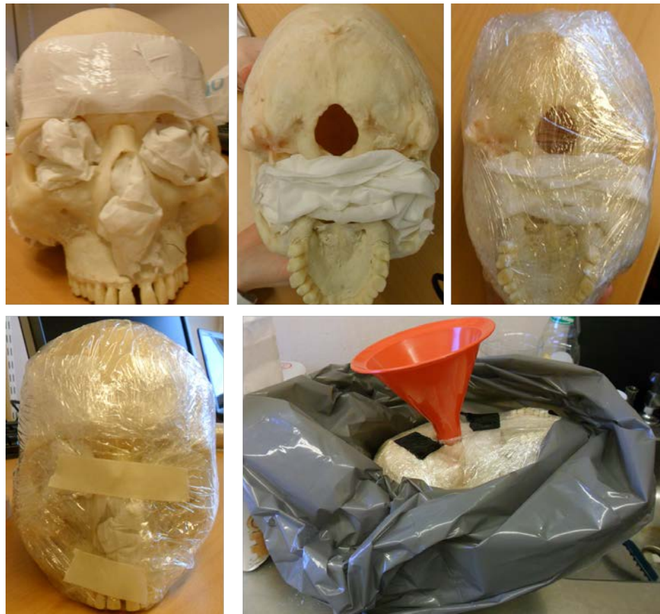
Figure A.2: Preparation of cranium before adding the agar solution.
