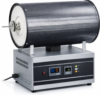
(a) Tubular furnace used for the oxidation experiments.
