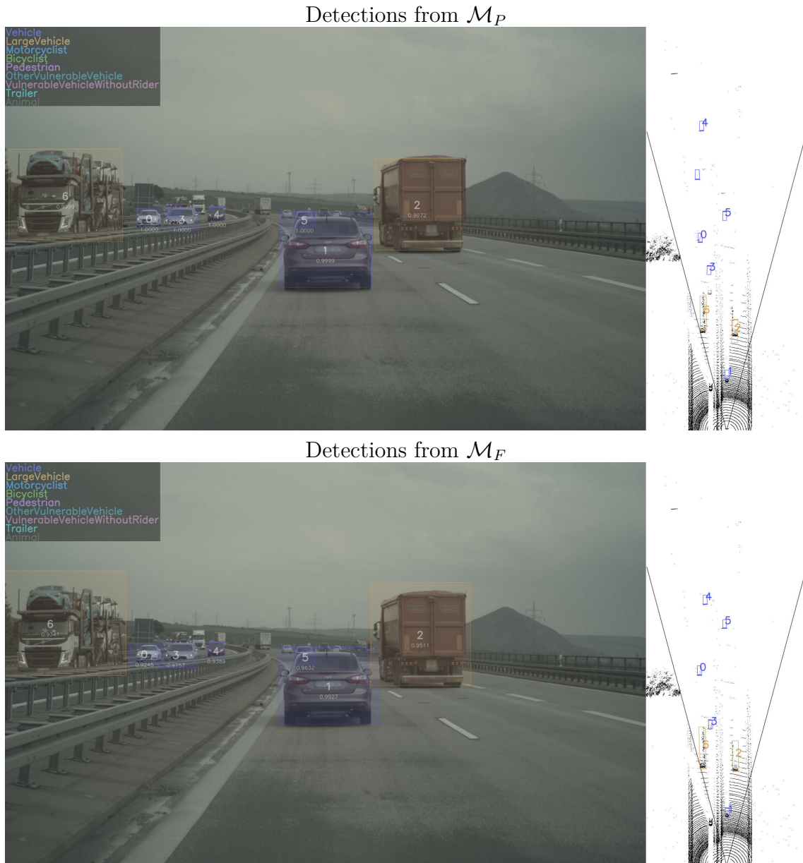
Figure 3.3: Example of sample where the discrepancy is small. There is only a small difference in depth between the matched detections and the largest difference are detections far away from the ego vehicle, meaning small discrepancy since the depth difference is relative.
