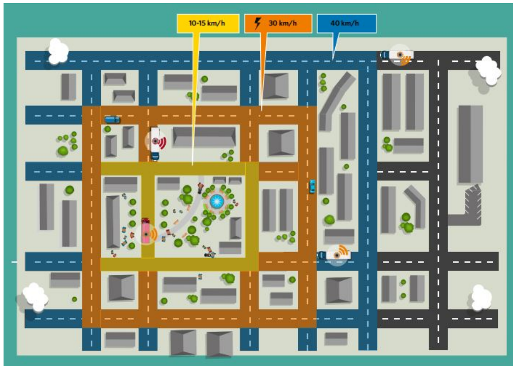
Figure 2.13: Conceptual illustration of how geofencing can work. (Swedish Transport Administration, 2018f)
