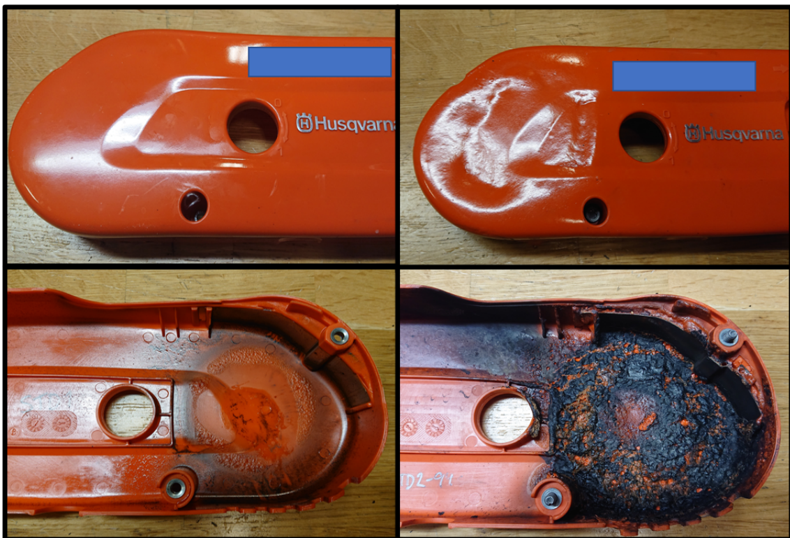
Figure 4.11: Two standard belt guards showed on outside and inside after heat resistance test. The left one was exposed to clutch slip for 1 time factor and the right one was exposed to clutch slip for 3.1 time factors.
