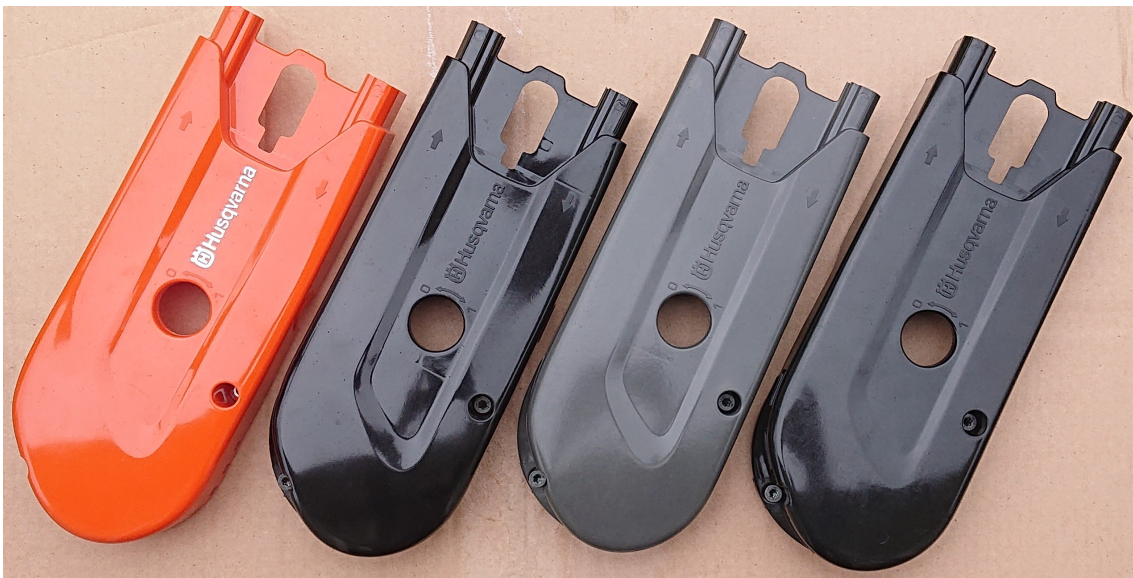
Figure 4.7: One belt guard in each of the materials. From left to right: DSM Standard Akulon, DSM Akulon RePurposed, Stora Enso DuraSense, Borealis Fibremod.
