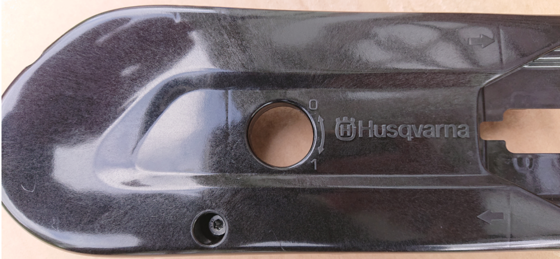
Figure 4.9: A Fibremod belt guard with visible streaks of glass fibres.
