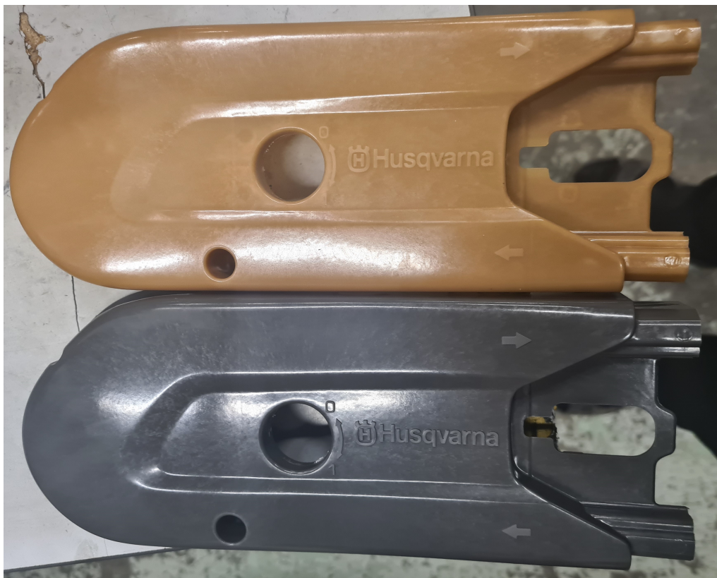
Figure 4.8: Two belt guards of the DuraSense Prime 30 Impact O. One uncolored as the material came from Stora Enso and one with grey color added.
