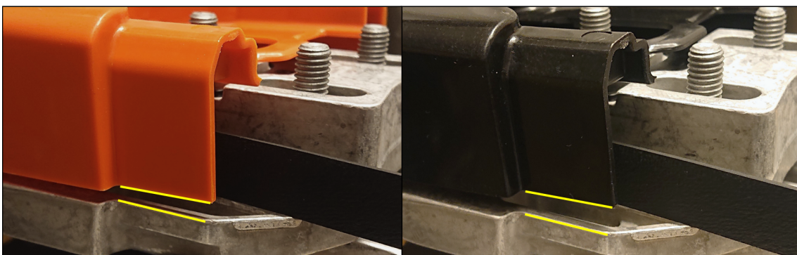
Figure 4.10: Two belt guards mounted to the crank case/cutting arm on a K770. To the left a standard belt guard and to the right a prototype made in Fibremod. The gaps considered are highlighted with the yellow lines.
