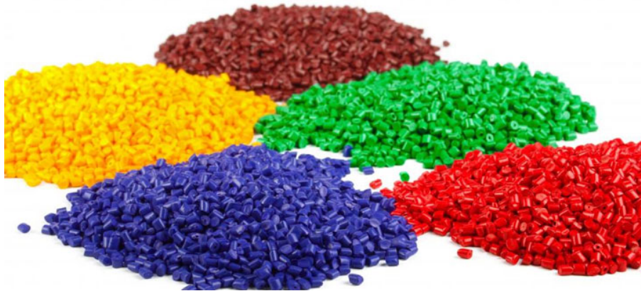
Figure 2.7: Typical plastic pellets, the raw material fed into an injection moulding machine. [17]
