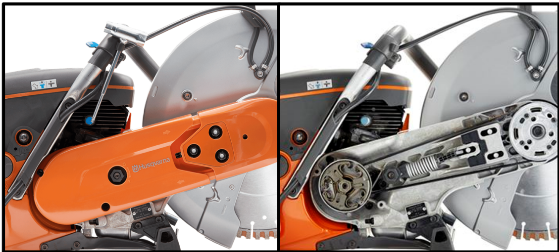
Figure 2.2: To the left, a Husqvarna K770 with the belt guard assembled. To the right, a K770 with the belt guard removed, revealing the drive belt and the centrifugal clutch behind it.
