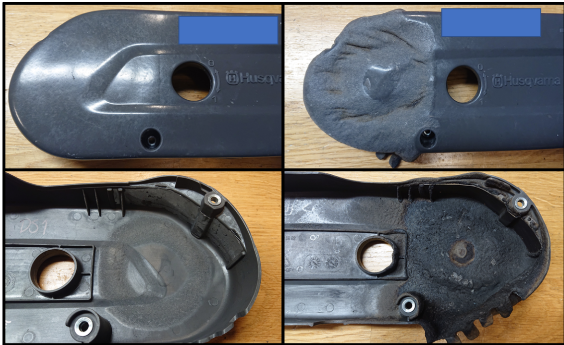
Figure 4.14: Two DuraSense belt guards showed on outside and inside after heat resistance test. The left one was exposed to clutch slip for 1 time factor and the right one was exposed to clutch slip for 3 time factors.
