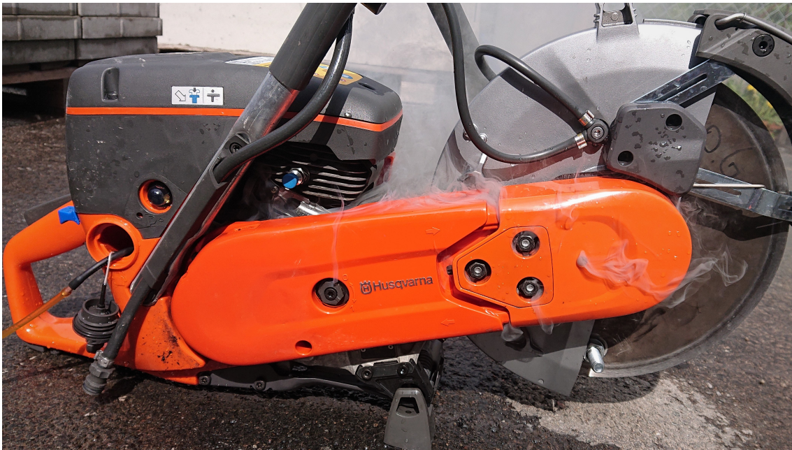
Figure 3.2: A K770 with a standard belt guard cooling down after extended clutch slipping.
