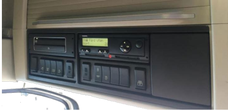
Figure 2.4 There is a panel above the windscreen on the driver's side. The panel consists of a tachograph which records the driver's speed and drive and rest times and electrical switches for extended truck functions.
