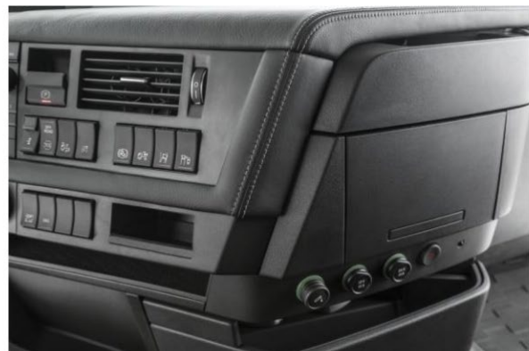
(b) The group of 16 electrical switches that are used for extended truck functions located on the right hand side of the steering wheel.
