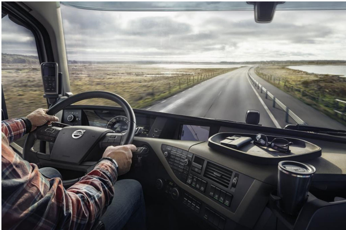
Figure 2.2 The Volvo FH truck interior. The truck interface consists of many controls and displays. There is instrument group in front of the steering wheel, a side display to the right of the instrument group and several controls such as buttons, switches and knobs. (Retrieved from Volvo Trucks Image and Film Gallery, n.d.)
