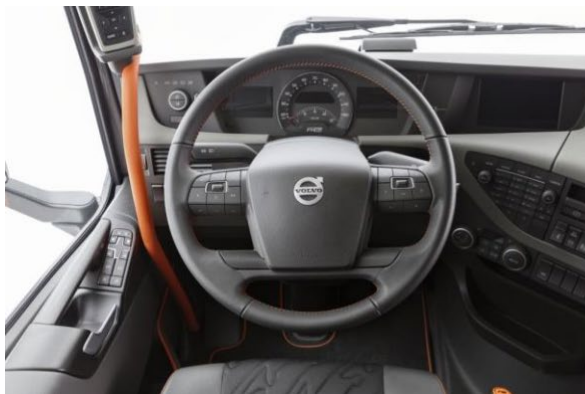
(a) The steering wheel with keypads. It contains buttons for Cruise Control, the infotainment system, phone etc.
