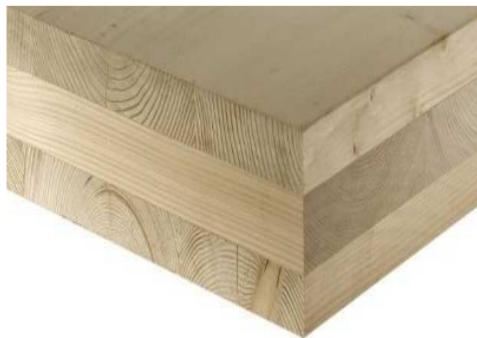
Figure 1.1: CLT plate. Figure from [14]
