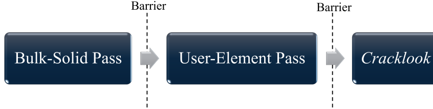
Figure 3.7: One solver cycle with the SMP multi-core implementation. The bulk-solid and user-element passes run in parallel across threads, LS-DYNA’s barrier between them guarantees that the bulk contributions to dm_a are in place before the user-element reads them. The cracklook routine runs once per cycle in serial and stages all cross-element data into history variables for the next cycle (synchronisation).
