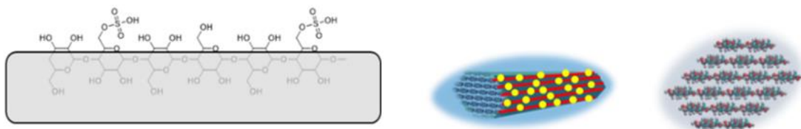
Figure 1. Overview of the structures of CNCs. From left to right: Illustration of crystal with sulphur half-esters on the surface. Illustration of CNC crystal with yellow dots representing the sulphate groups. Hexagonal cross-section of the CNC crystals.
