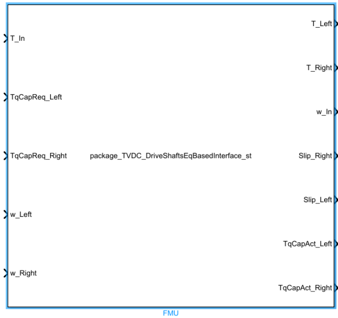
Figure 3.19: TVDC driveline Functional Mock-up Unit (FMU) imported in Simulink
