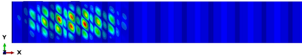
Figure 3.10: First buckling mode for girder G7A
