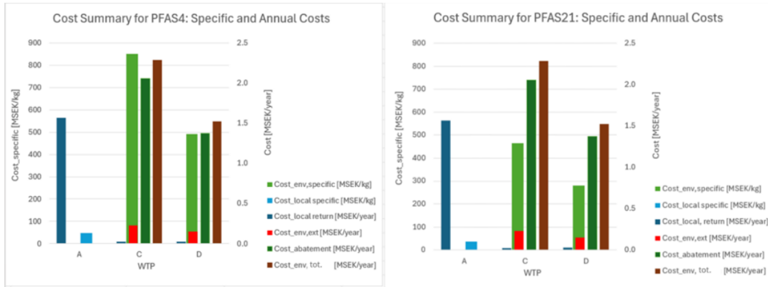
Figure 5: Economic summary of PFAS4- (left) and PFAS21- (right)-related costs for facilities A, C and D. Left axis shows specific costs in MSEK/kg (light green and light blue bars). Right axis shows annual total costs in MSEK/year (brown, red, dark blue, and dark green bars).
