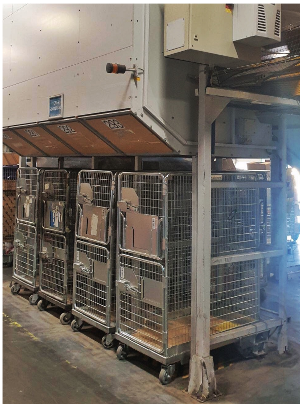
Figure 16. The load carriers that parcels are dropped into at PostNord's sorting facility.
