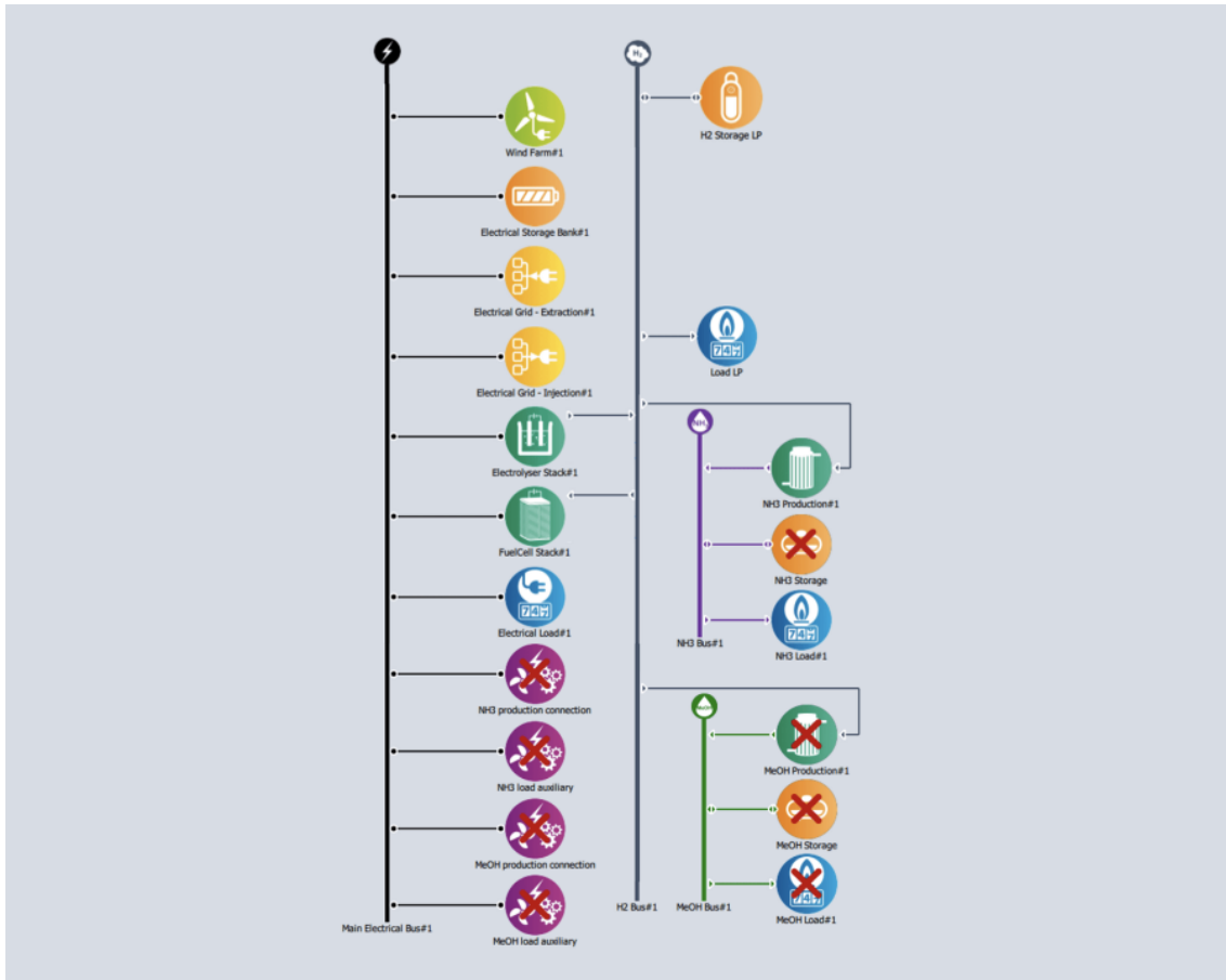
Figure 3.4: Overview of the system architecture in Odyssey.
