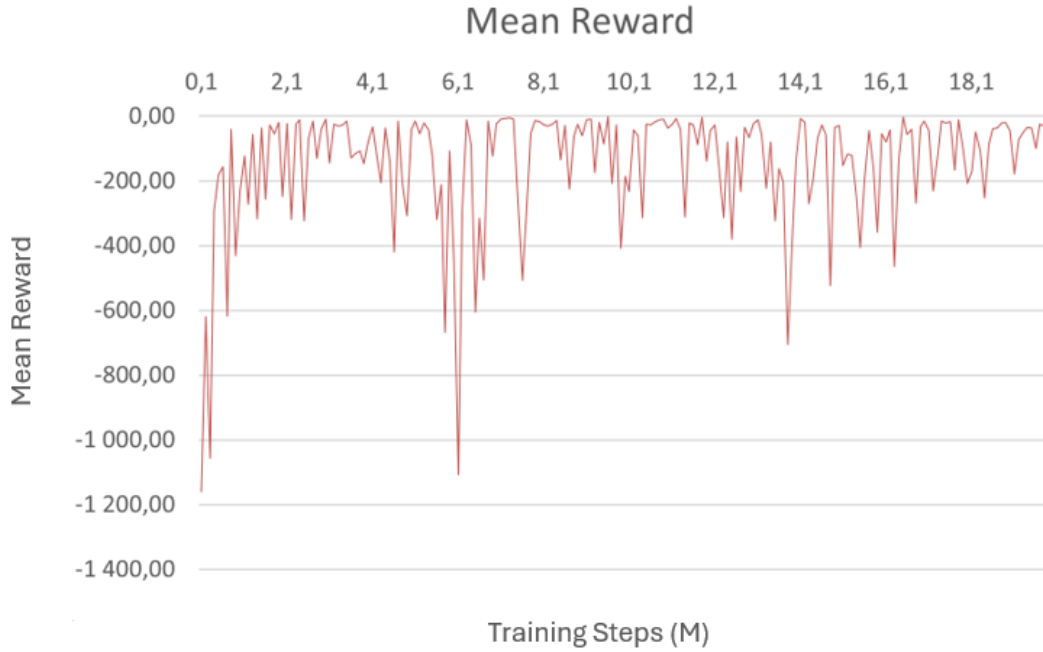
Figure 4.2: Mean cumulative reward on 10 holdout seeds at every 100,000-step checkpoint over 20 million training steps (Experiment 2, \gamma = 0.98 ).
